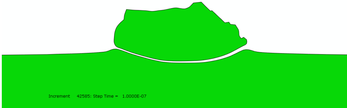
Figure 15: FEA of Aluminum particle at 0.1 ms after the impact.
