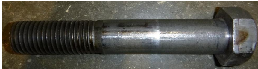
(c) No bending in bolt
