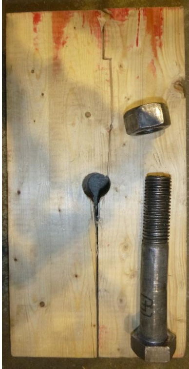
(a) Splitting failure
