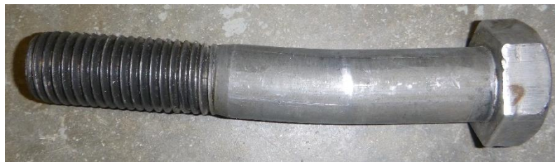
(c) Slight bend in bolt
