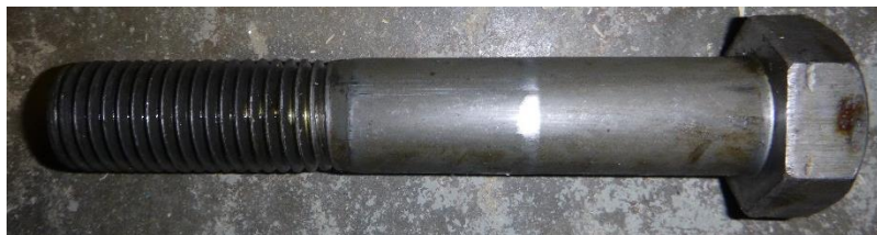
Figure 3.3: 25.4 mm ASTM A307 Grade A hex bolt
