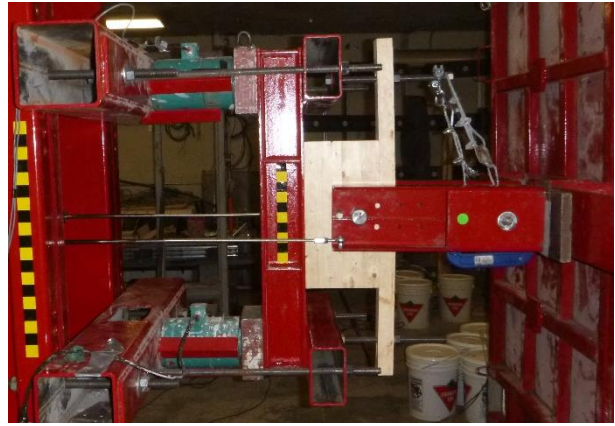
(b) Perpendicular to the grain connection designed to fail in Mode I
