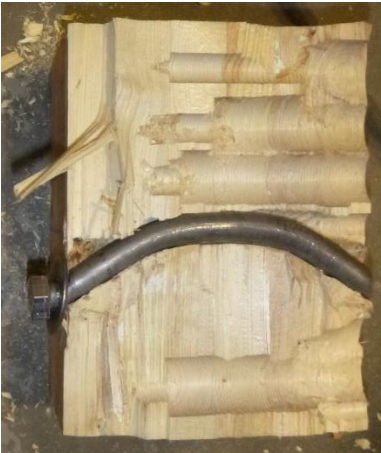
(a) Specimen cut open to show deformed shape of bolt
