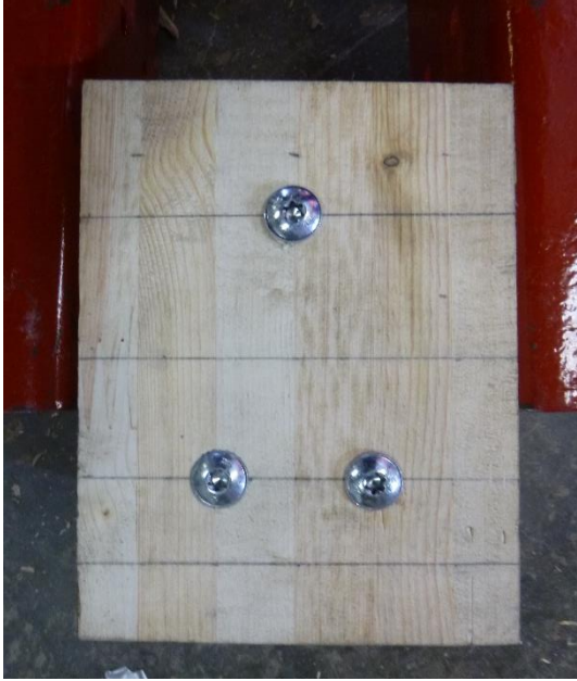
(a) Self-tapping screw reinforcement configuration
