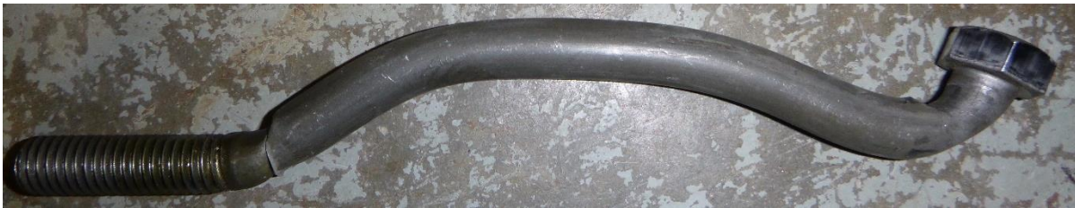
(c) Deformed shape of bolt and shear failure on nut side
