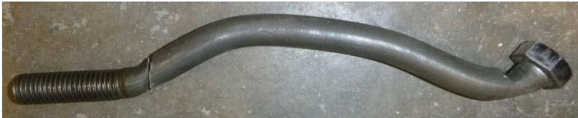
(c) Deformed shape of bolt and shear failure on nut side
