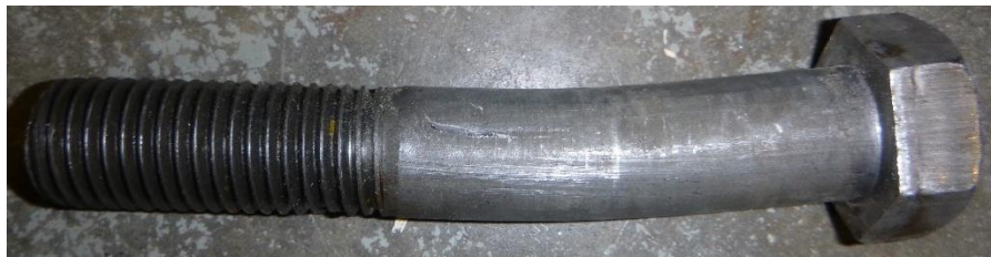
(c) Slight bending in bolt
