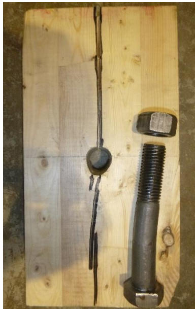
(a) Splitting failure
