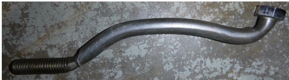
(c) Deformed shape of bolt and shear failure on nut side
