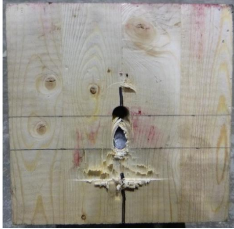
(a) Static test – bolt shear failure
