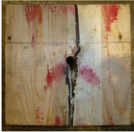
(a) Unreinforced – splitting failure
