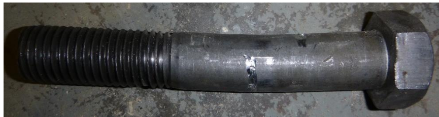
(c) Slight bending in bolt
