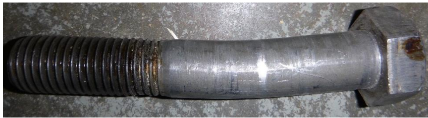
(c) Slight bending in bolt
