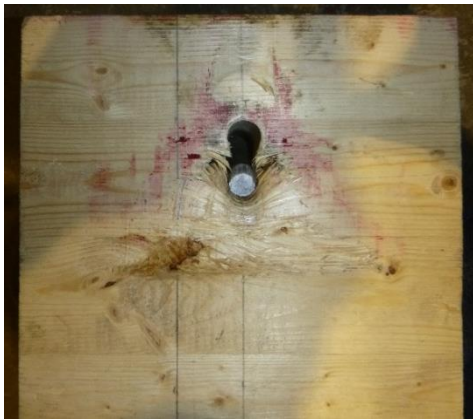
(a) Specimen after testing, bolt head side
