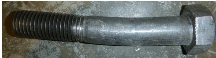
(c) Slight bending in bolt
