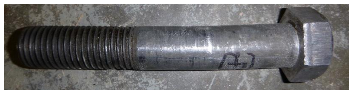
(a) Connections designed to fail in Mode I: slight deformation in 25.4 mm bolt
