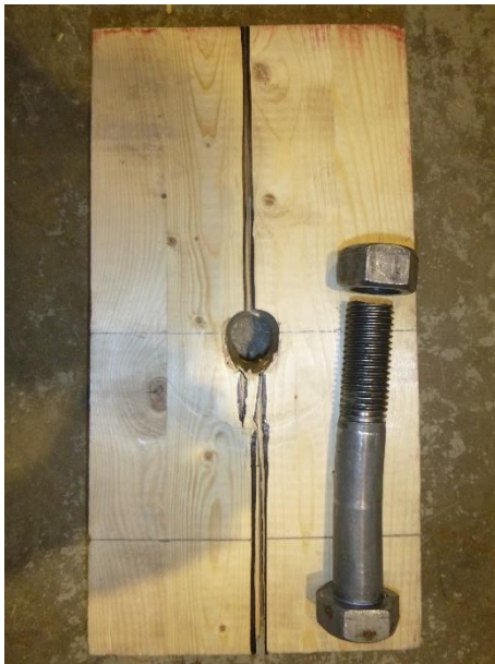
(a) Splitting failure
