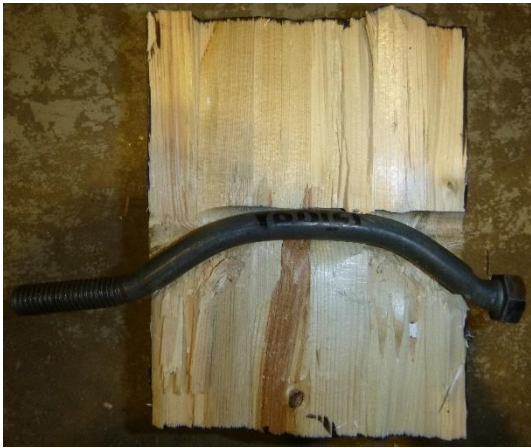
(a) Inside of split specimen
