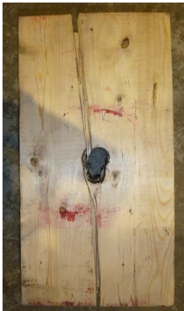
(a) Splitting failure
