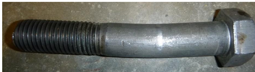
(c) Slight bend in bolt
