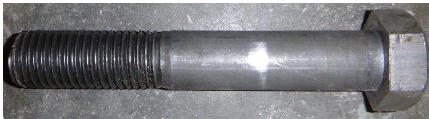
(c) No bending in bolt
