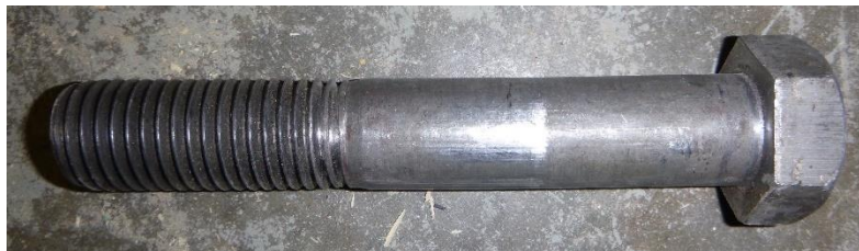
(c) No bending in bolt
