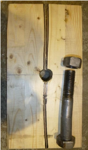
(a) Splitting failure
