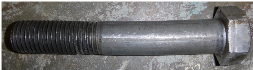
(c) No bending in bolt
