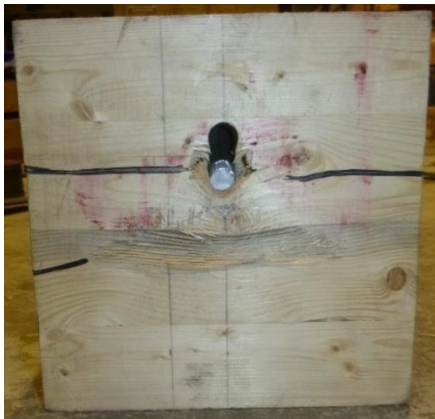
(a) Specimen after testing, bolt head side
