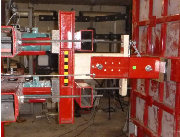
(a) Parallel to the grain connection designed to fail in Mode I
