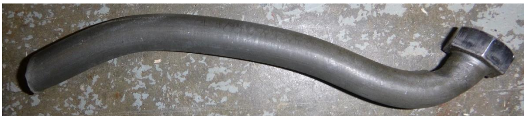
(d) Deformed shape of bolt and shear failure on nut side
