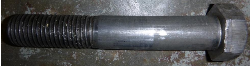
(c) No bending in bolt
