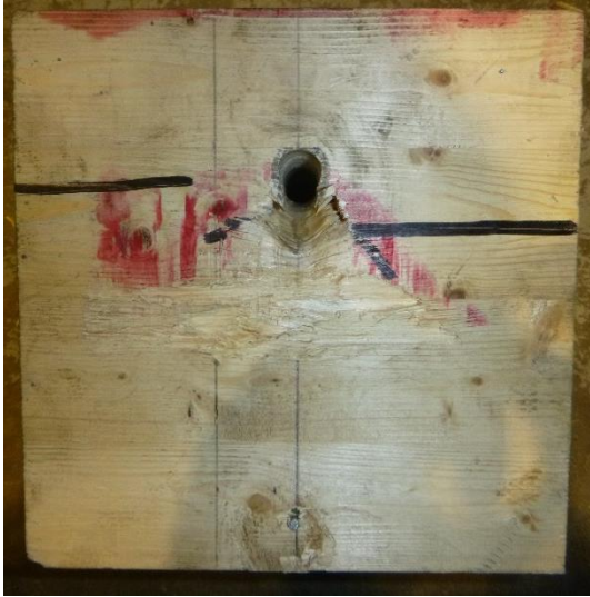
(a) No splitting failure
