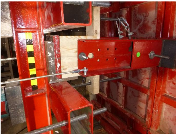
(c) Parallel to the grain connection designed to fail in Mode III
