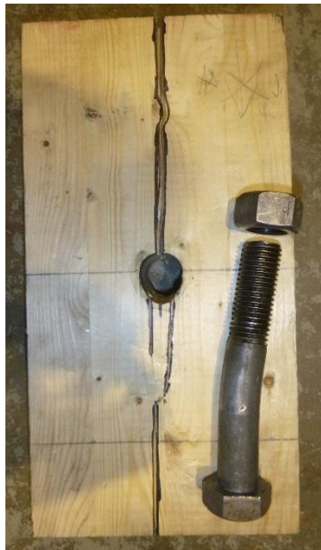
(a) Splitting failure
