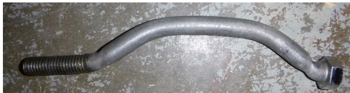
(b) Connections designed to fail in Mode III: bending in 12.7 mm bolt
