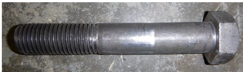
(c) No bending in bolt
