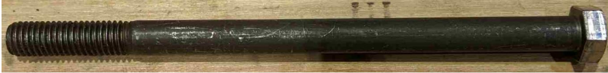
Figure 3.6: 12.7 mm ASTM A307 Grade A hex bolt
