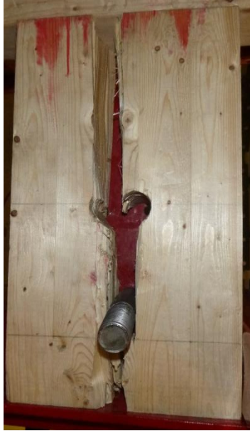
(a) Unreinforced – splitting failure
