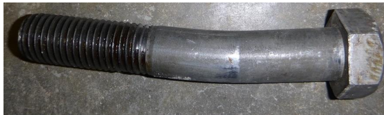
(c) Slight bend in bolt
