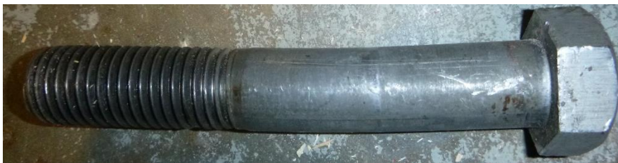
(c) No bending in bolt
