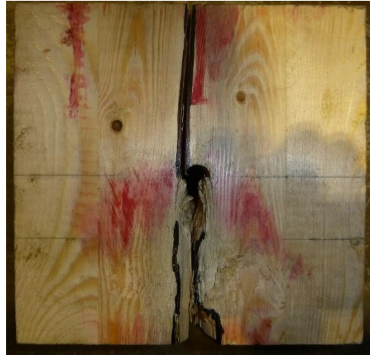
(b) Splitting failure
