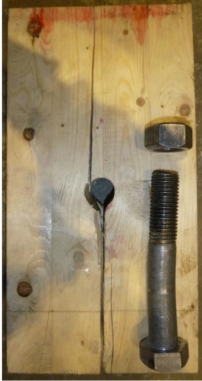
(a) Splitting failure
