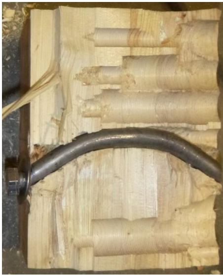
(a) Specimen cut open to observe crushing in wood
