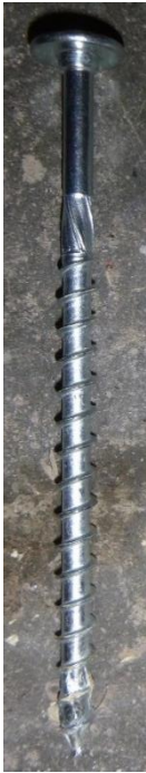
Figure 3.7: 8x120 mm Heco-Topix self-tapping screw
