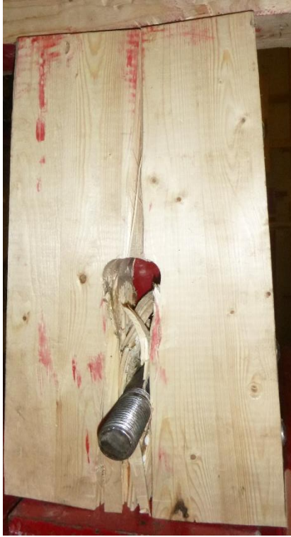
(a) Ultimate failure in screw withdrawal
