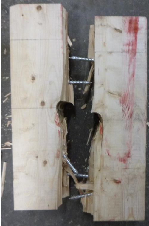
(a) Ultimate failure in screw withdrawal
