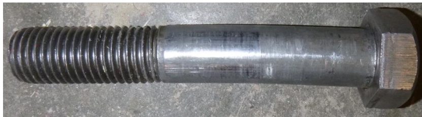
(c) Slight bending in bolt
