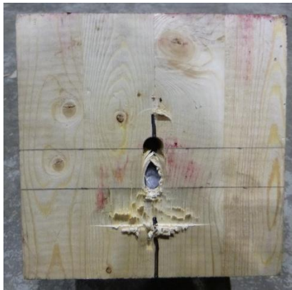
(a) Specimen after testing, bolt head side
