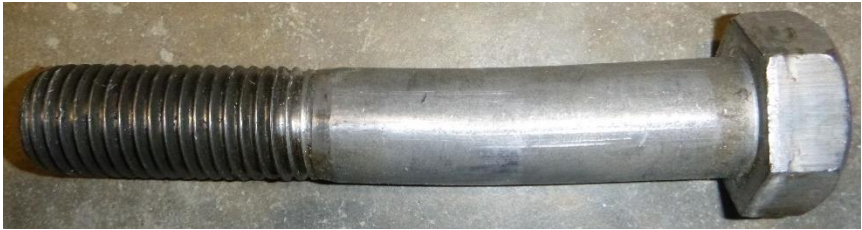
(c) Slight bend in bolt
