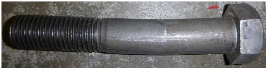
(c) Slight bending in bolt
