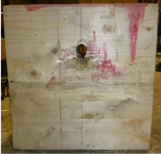
(a) No splitting failure
