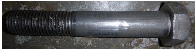
(b) 25.4 mm bolt after testing
