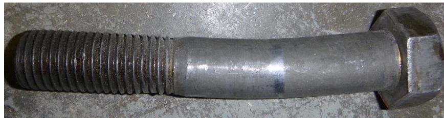
(c) Slight bending in bolt
