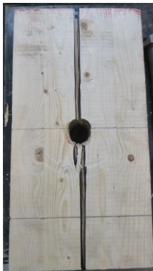
(a) Splitting failure
