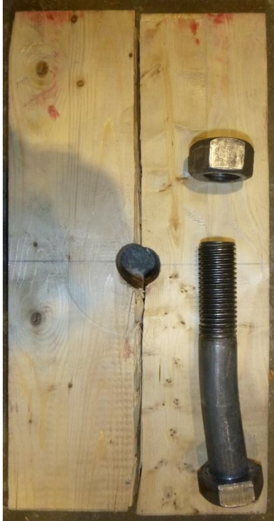
(a) Splitting failure
