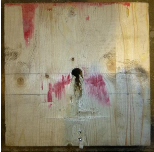
(a) No splitting failure
