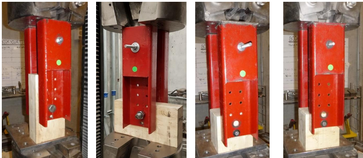
(a) Mode I parallel to the grain
