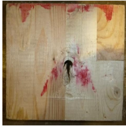
(b) Reinforced – bolt shear failure
