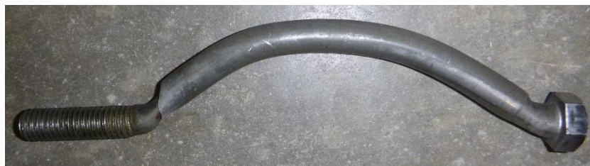
(c) Deformed shape of bolt and shear failure on nut side
