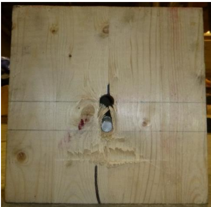
(a) Specimen after testing, bolt head side
