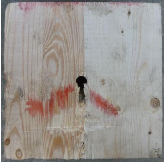
(a) No splitting failure
