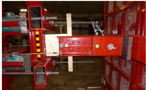
(d) Perpendicular to the grain connection designed to fail in Mode III
