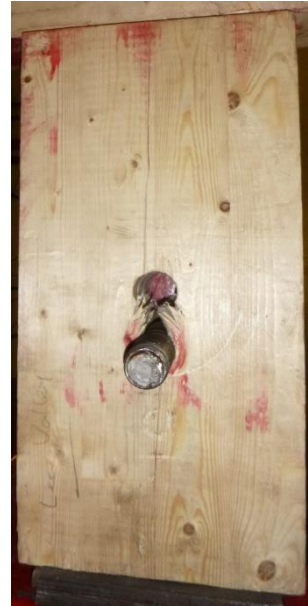
(b) Reinforced – plastic deformation
