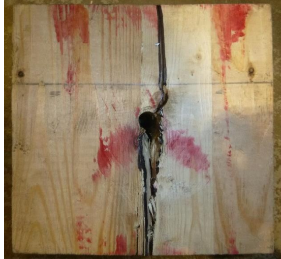
(b) Splitting failure
