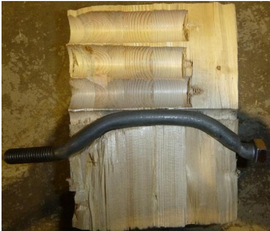
(a) Specimen cut open to observe crushing in wood
