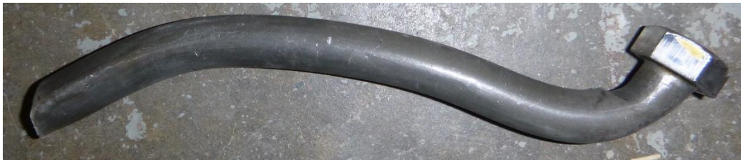
(c) Deformed shape of bolt and shear failure on nut side
