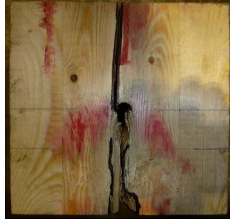
(b) Dynamic test – splitting failure
