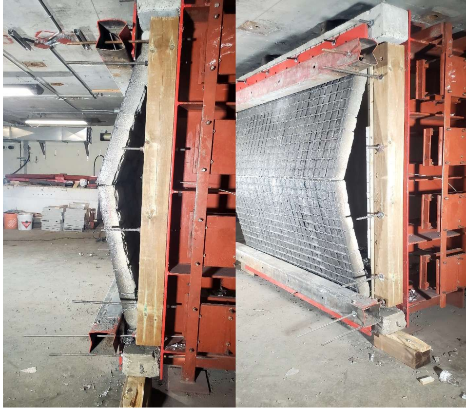
Figure 4.49. Wall-4 split into two halves after shot 5 with no release of debris
