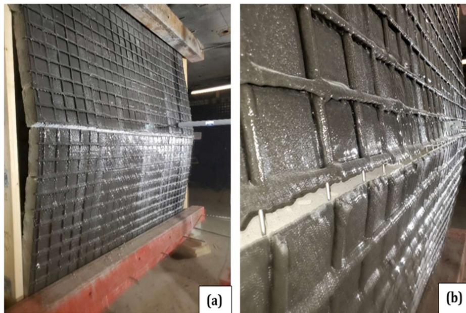
Figure 4.8. (a) Wall-1 split into two equal parts at mid-height after shot 4 (b) Mortar failure and SS304 strands necking point after shot 4
