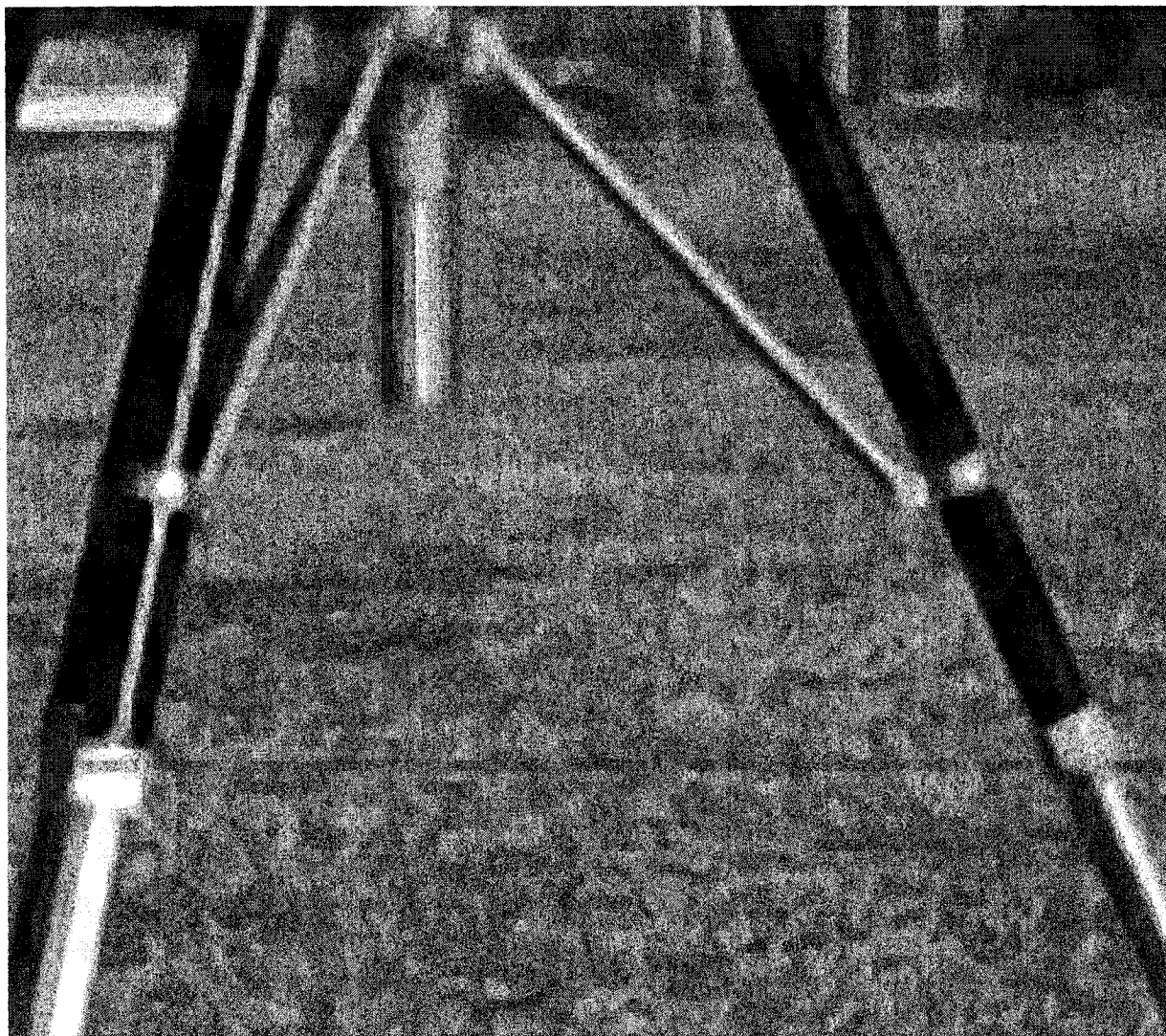
Fig. 5.5 Up-sampling of the tripod of the cameraman image by a factor of 25 using the proposed approach for 300 iterations and with \lambda = 0.15 .
