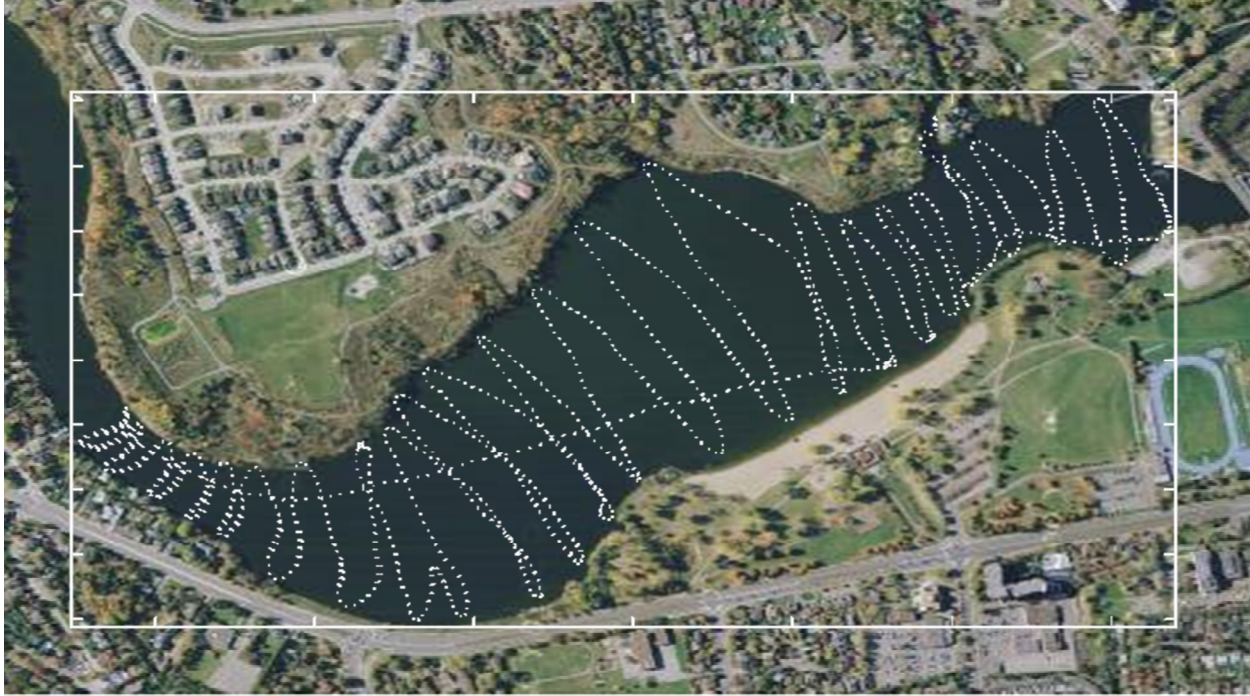
Figure 5-1: Path Taken by Boat Equipped with ADCP (Kheradmand et al. 2015)
