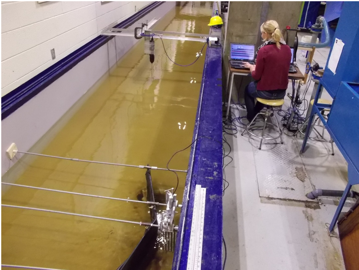
Figure 4-6: Overall Flume Testing Setup
