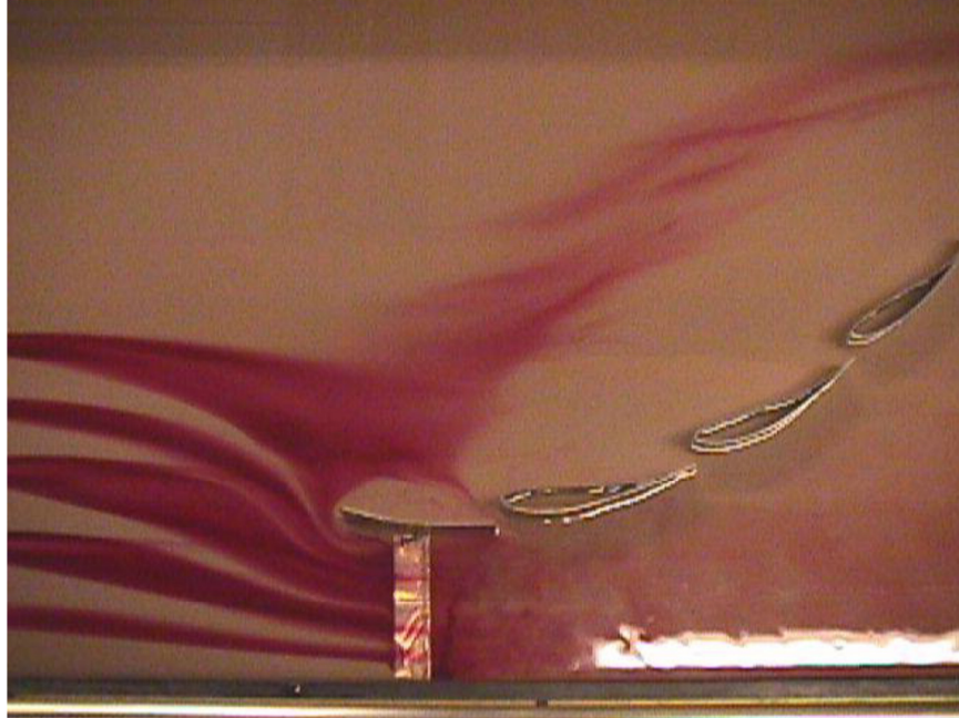
Figure 2-12: Multiple Hydrofoil Diffuser Drawing in Upstream Flow - Plan View (Kirke 2006)
