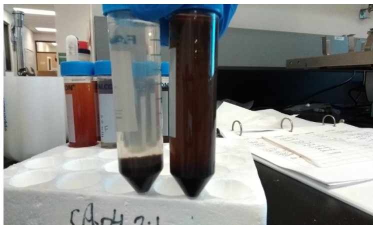
Fig. S28: Difference in the aggregation and coagulation of the native (left) and post-irradiated (right) ferrihydrite coprecipitated with C/Fe ratio of 0.5. The picture was taken at the end of the experimental period (25 days) of exposure to Shewanella putrefaciens CN32.
