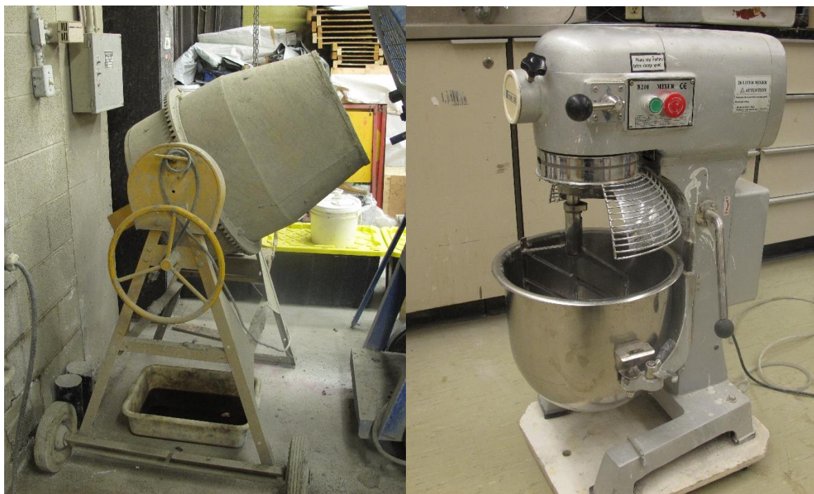
Figure A-2. (Right) Food mixer for preparing small volume batches of CPB used in pressure cell experiments; and (Left) Concrete mixer for preparing large volume batches of CPB used in column experiments.
