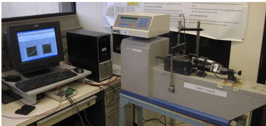
Figure A-6. Direct Shear test machine used to determine shear strength properties of CPB samples
