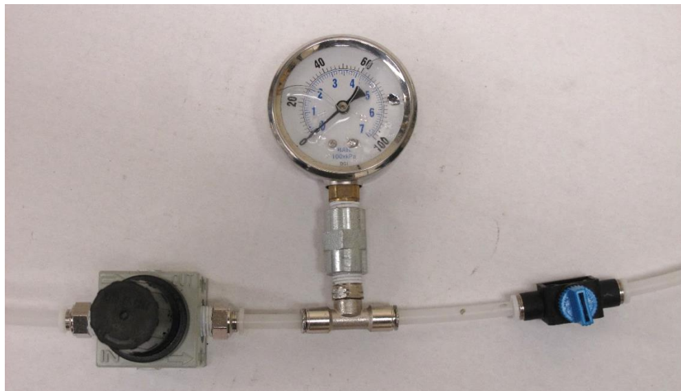
Figure A-19. Regulator (600 kPa), pressure gauge and valve used for pressure control and load application in load cell experiments
