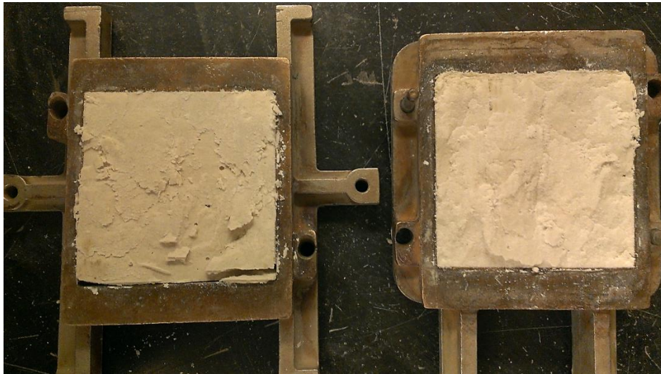
Figure A-9. After performing direct shear test on the cured under stress sample (Silica tailings, 0.31m/h, undrained and 150 days).
