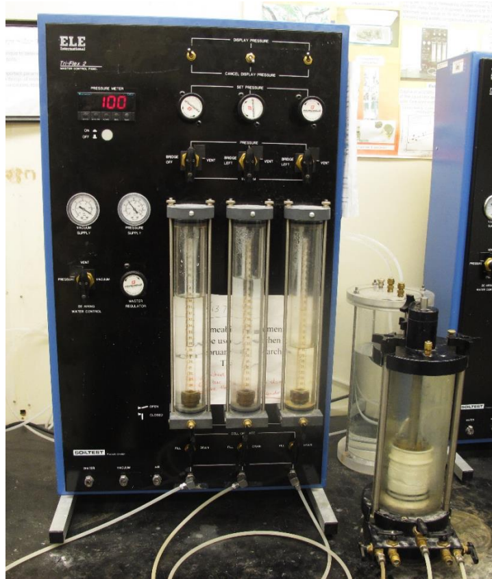
Figure A-7. ELE hydraulic conductivity apparatus used to measure saturated hydraulic conductivity of CPB samples
