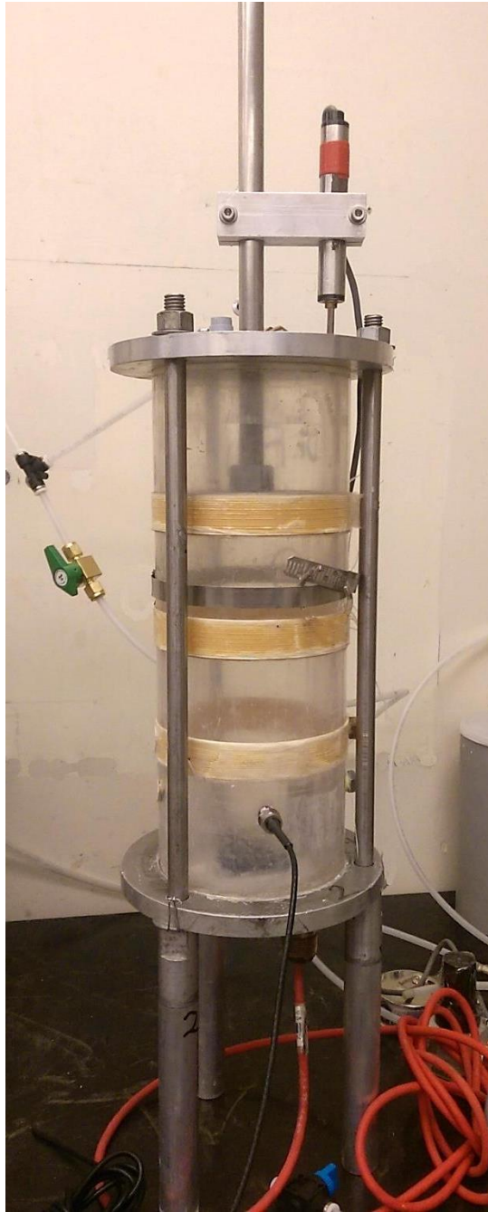
Figure A-17. Curing under stress load cell used in monitoring programs
