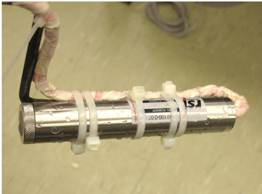
Figure A-15. Standard vibrating wire piezometer model WP2100, RST, 70 kPa capacity used in high column experiments
