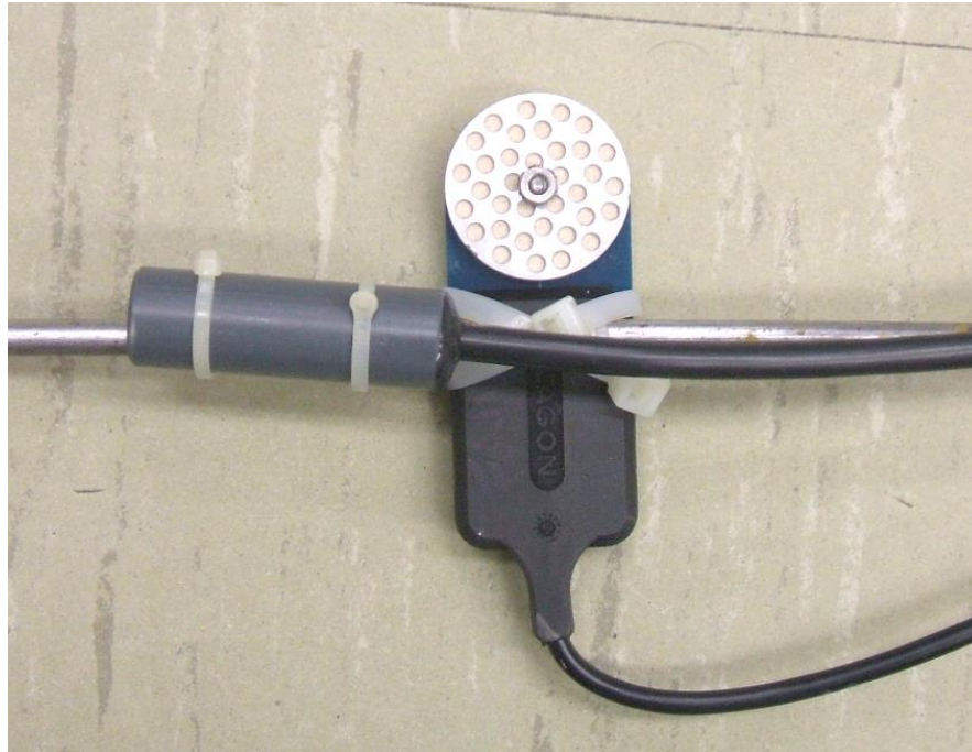
Figure A-14. Temperature sensor (model: TH-T, Roctest) and suction meter (model: MPS-1, Decagon) used in column experiment
