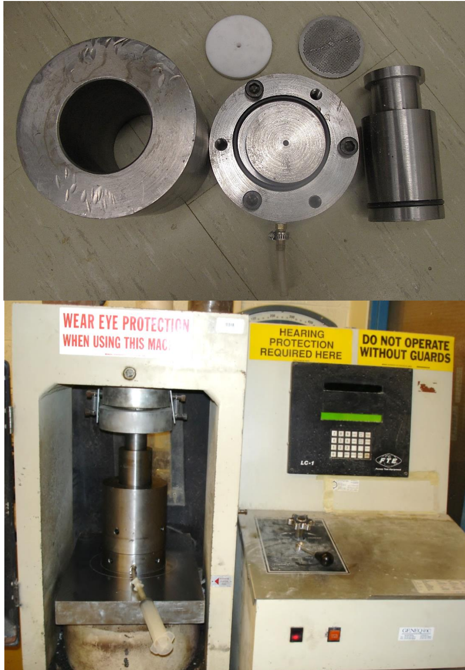
Figure A-22. CPB pore water squeezer designed and manufactured at the University of Ottawa (top); and squeezer apparatus under hydraulic pressure jack during the pore water extraction (bottom)
