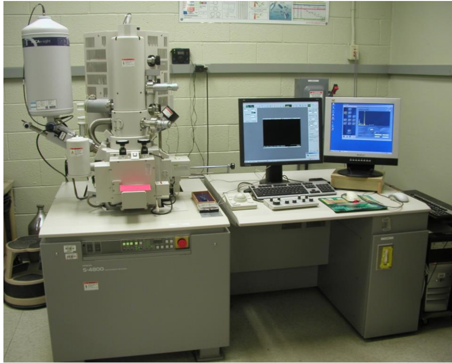
Figure A-24. SEM equipment (Hitachi S4800) at National Research Council of Canada (NRC) used to perform SEM analysis on samples in column experiments
