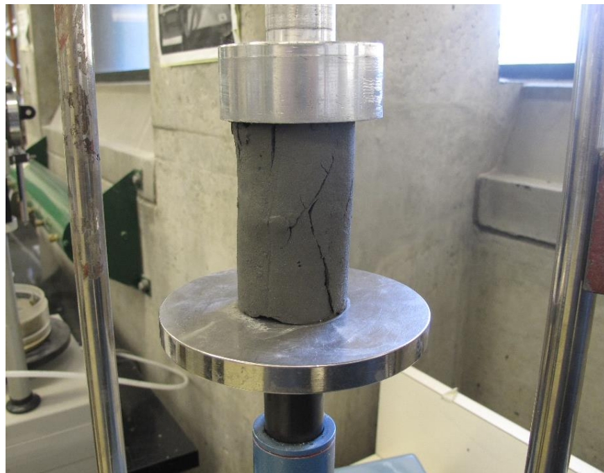
Figure A-8. Performing UCS test on CPB sample prepared with zinc tailings
