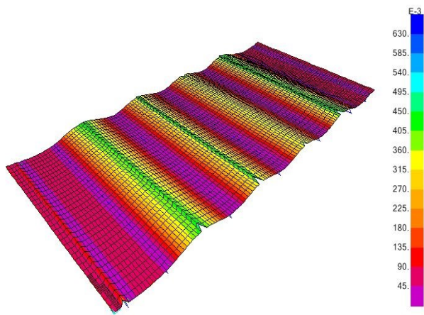
Roof assembly 6', deflection (in), 90 psf distributed load
