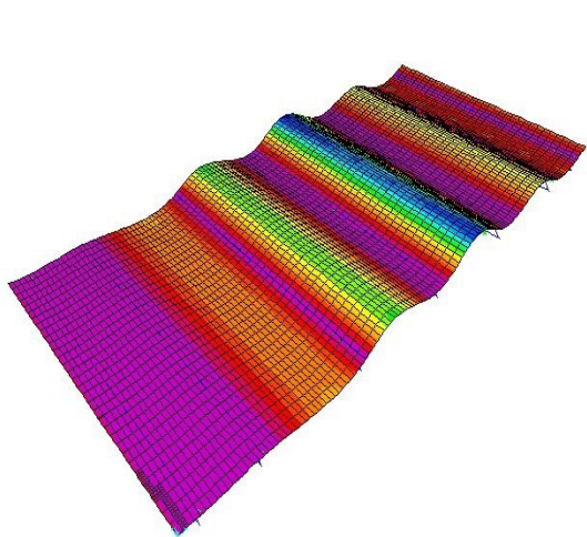
Roof assembly 7'6", deflection (in), 90 psf point load
