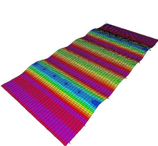
Steel deck deflection (in), 120 psf uniform
