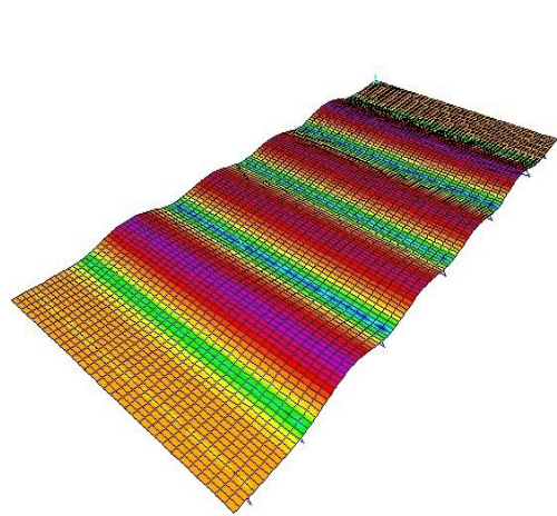
Steel deck moment (lb-in), 120 psf uniform load
