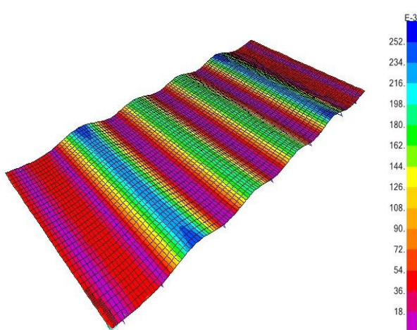
Roof assembly 6', deflection (in), 60 psf point load uniform
