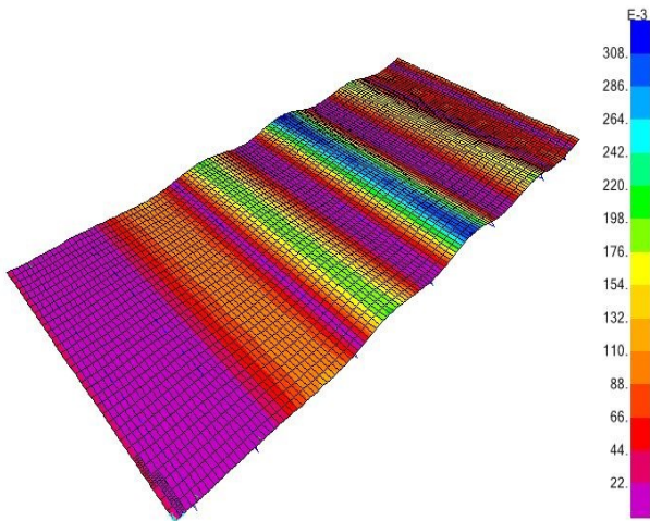
Roof assembly 7'6", deflection (in), 60 psf point load
