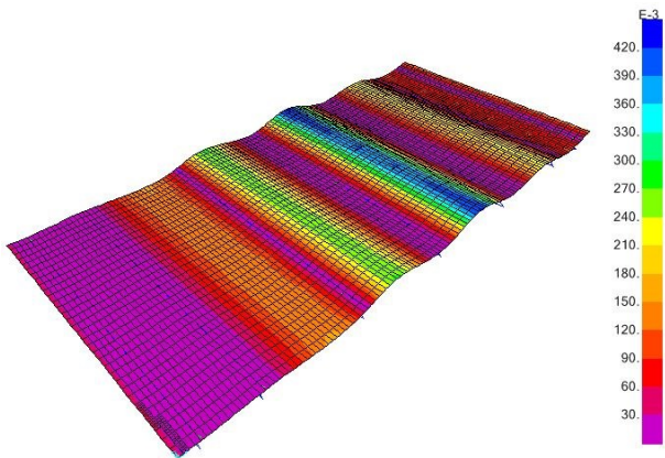
Roof assembly 7'6", deflection (in), 75 psf point load
