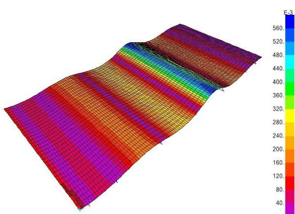
Roof assembly 9'6", deflection (in), 60 psf point load
