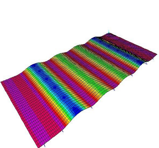
Steel deck deflection (in), 135 psf uniform
