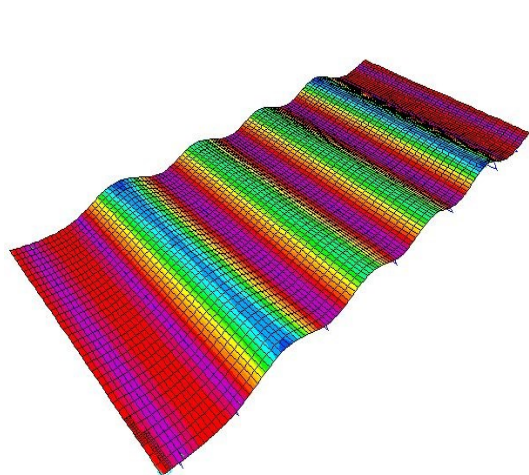
Roof assembly 6', deflection (in), 105 psf point load
