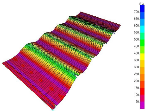
Roof assembly 6', deflection (in), 105 psf distributed load
