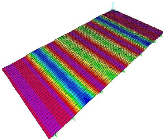
Steel deck deflection (in), 45 psf uniform load
