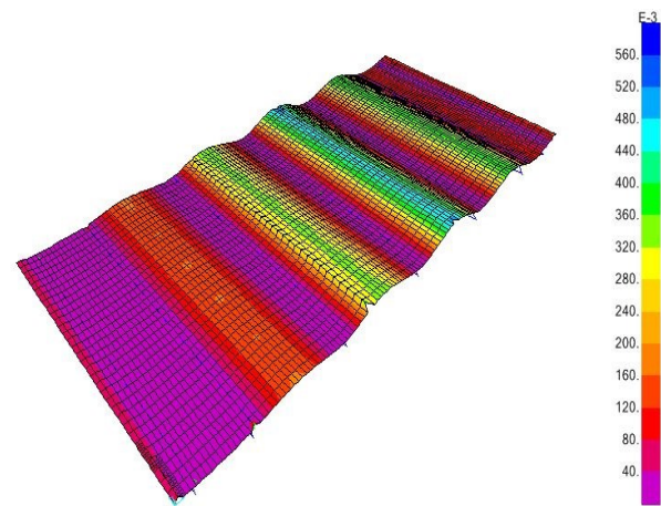
Roof assembly 7'6", deflection (in), 60 psf distributed load
