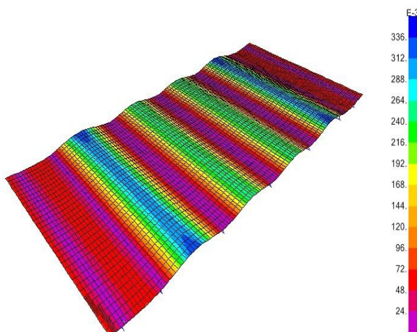
Roof assembly 6', deflection (in), 75 psf point load uniform
