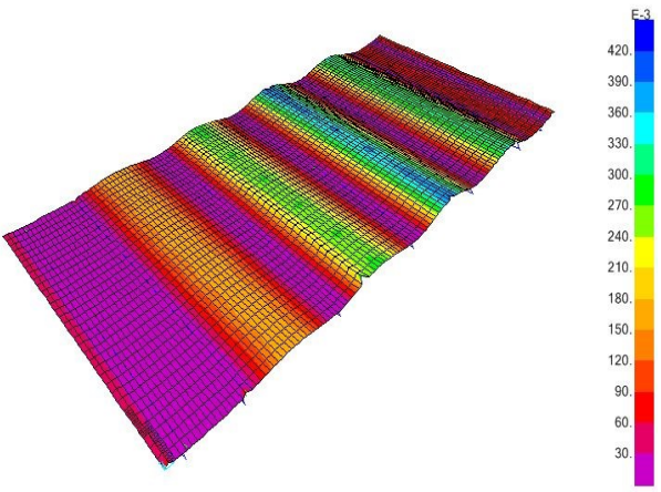
Roof assembly 7'6", deflection (in), 45 psf distributed load
