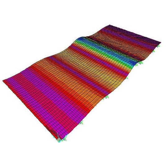
Roof assembly 9'6", deflection (in), 75 psf point load
