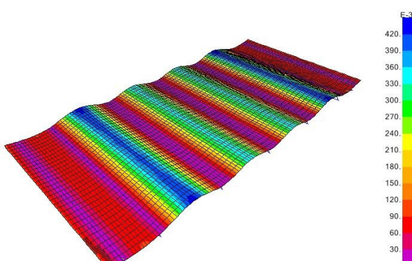
Roof assembly 6', deflection (in), 90 psf point load uniform
