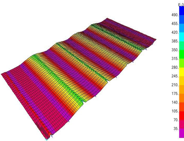
Roof assembly 6', deflection (in), 75 psf distributed load
