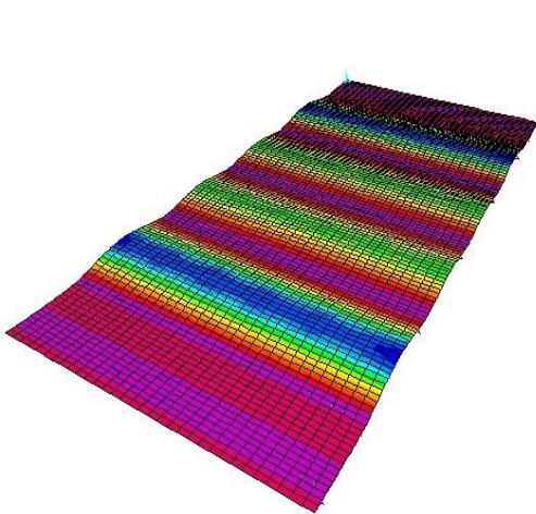
Steel deck deflection (in), 90 psf uniform load
