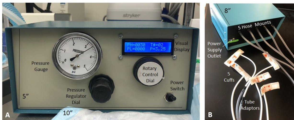
Figure 6. Automatic ischemic conditioning cuff pump. (A) Front view with labels and dimensions. Rotary control dial controls the inflation time in seconds (“PH” = pressure high), deflation time in seconds (“PL” = pressure low) and number of cycles (“T#” = trial number). Pressure regulator dial controls the pressure gauge. Actual pressure generated is displayed in the visual display (“P” = pressure in psi). Current settings: 30 seconds remaining of inflation, 2 cycles remaining and 3.25 psi cuff pressure. (B) Back view displaying the 5 inflatable cuffs attached to the pump with labeled parts.
