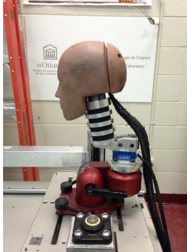
Figure 4: Hybrid III head attached to unbiased neck form and sliding table
