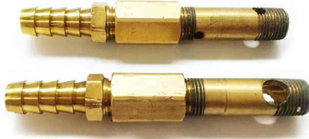
Figure 3.13: End fixtures manufactured using off-the-shelf plumbing products.
