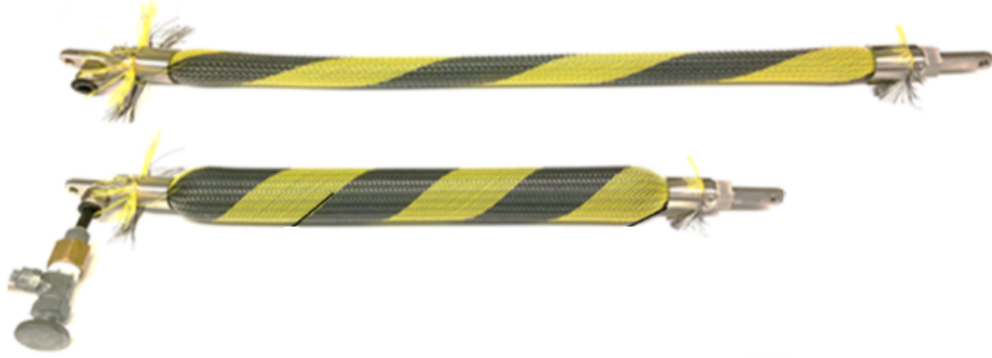
Figure 3.1: Deflated (top) and inflated (bottom) PAM [4].
