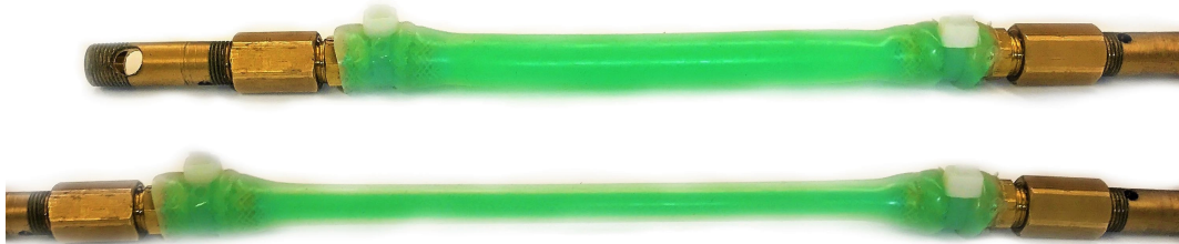
Figure 1.2: SC prototype in its resting (top) and stretched (bottom) configuration.
