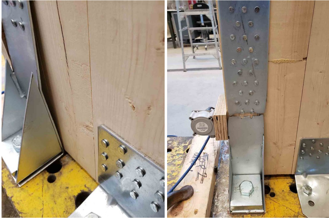
Figure 6-20: Shearwall test #11: (a) before failure (b) after failure
