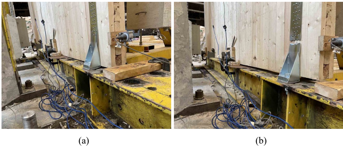
Figure 6-11: Shearwall test #2: (a) before failure (b) after failure
