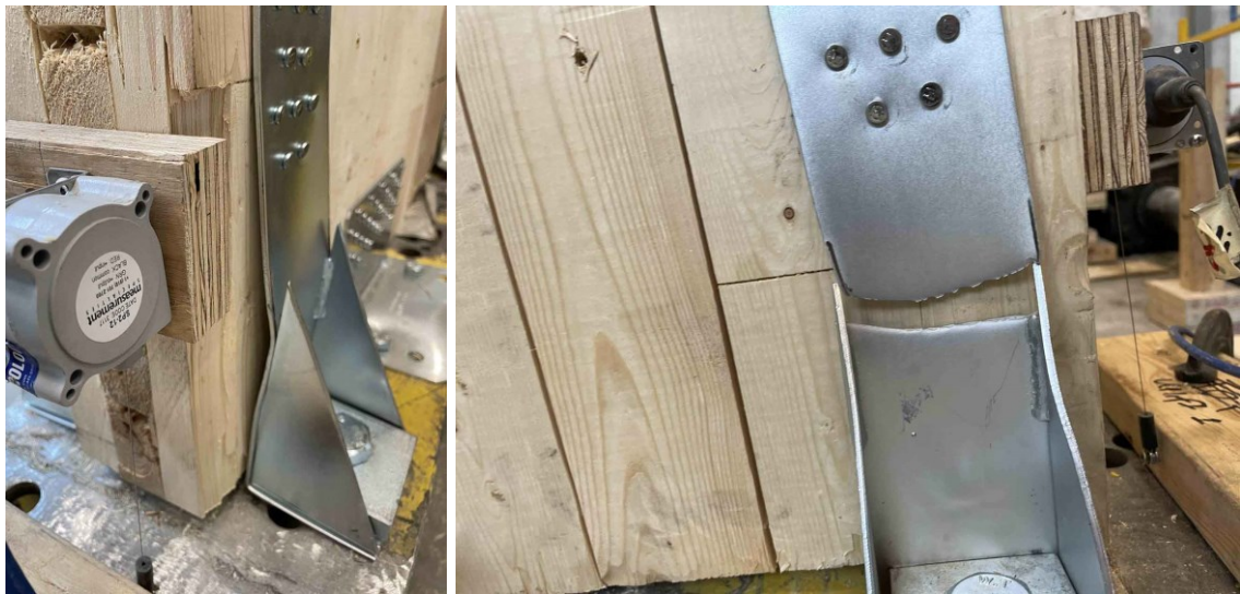
Figure 6-21: Shearwall test #12: (a) before failure (b) after failure
