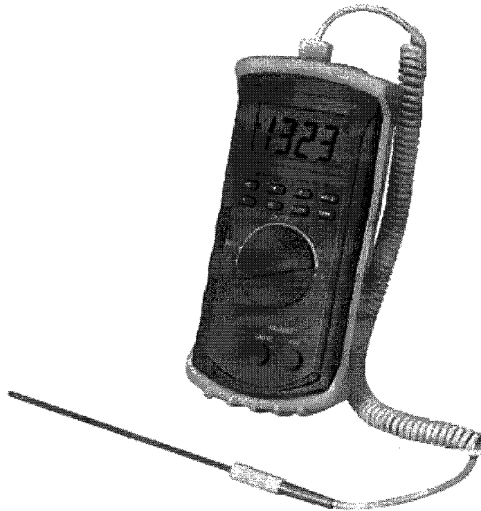
Figure 22 – Omega digital thermometer with removable probe (Image altered from Omega Inc. promotional data sheet)
