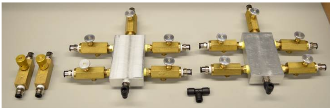
Figure 3.44: Demonstrator Rig Manifolds and Shut-Off Valves
