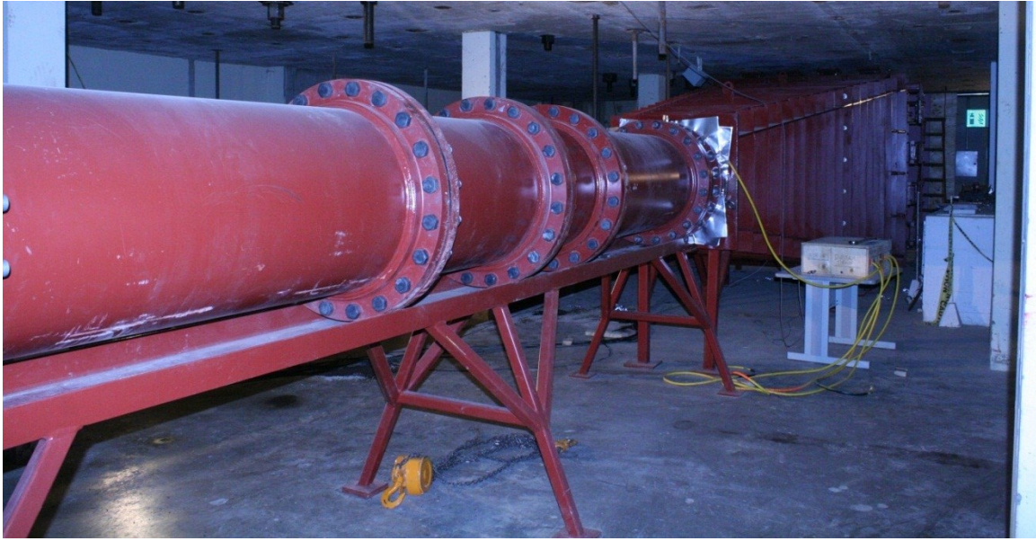
Figure 3-10: Driver Section, Diaphragms, and Expansion Section of Shock Tube
