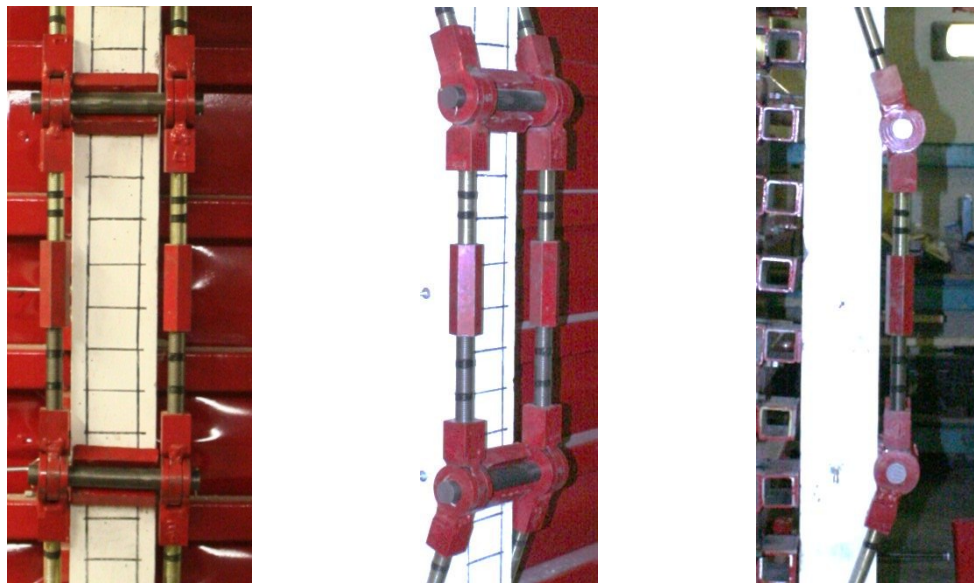
b) Tension Brace Turnbuckle Installed on Column
