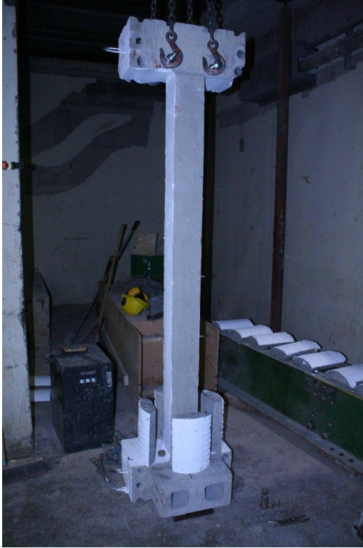
a) Wedges Placed for Installation
