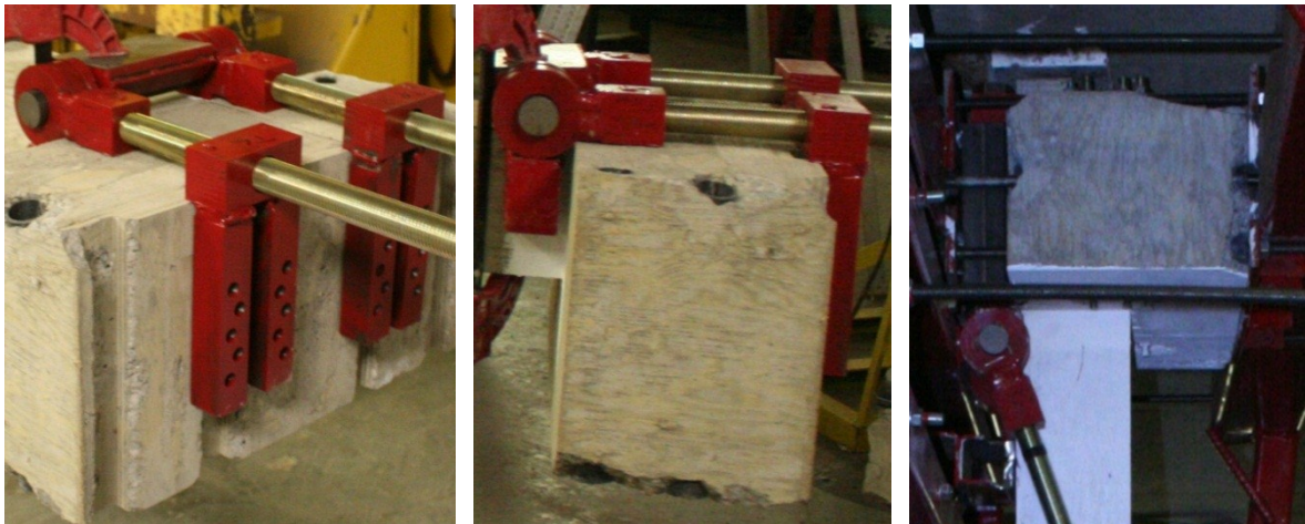
b) End Hinge and Bearing Connector Installed on Column
