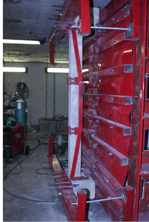
b) Vertical Members and Bearing Plates
