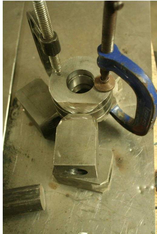
b) Hinge Coupler Prior to Welding
