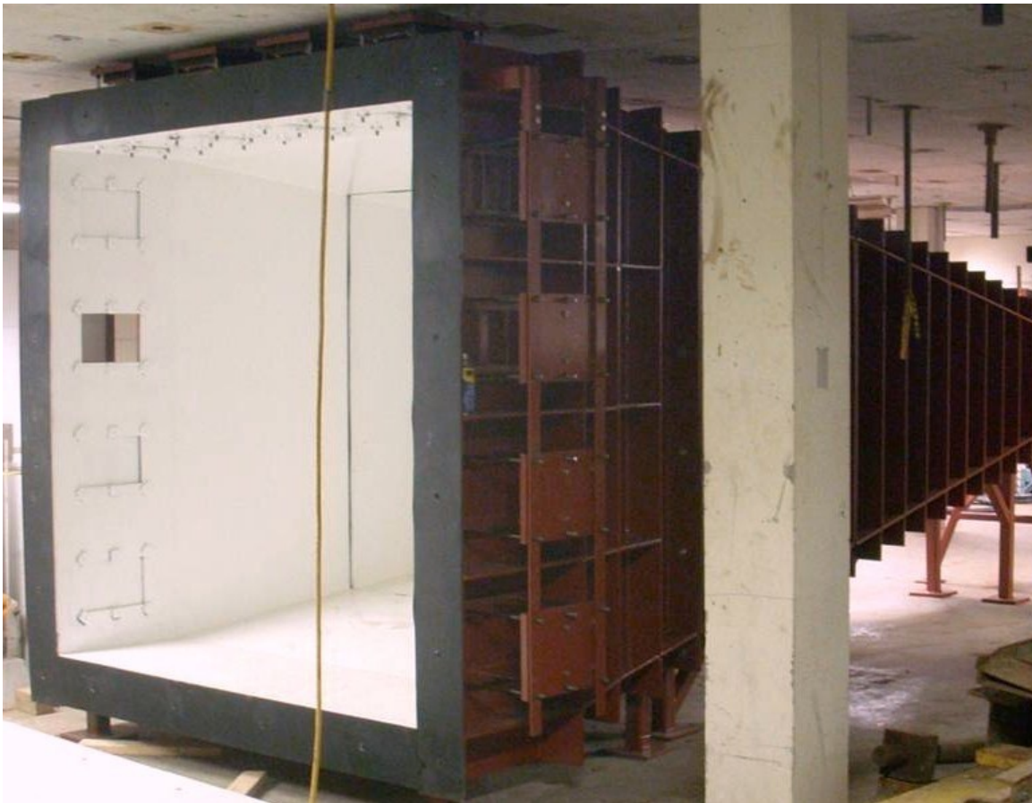
Figure 3-11: Shock Tube Opening, Test Frame and Expansion system
