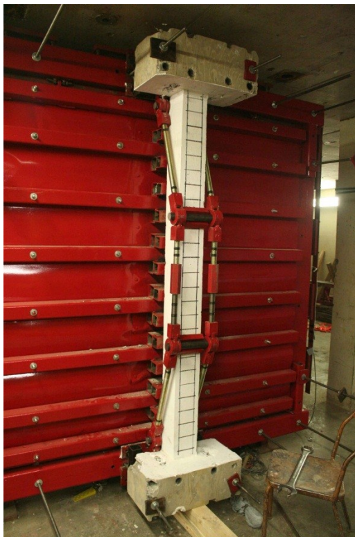
c) Completed Brace Installation
