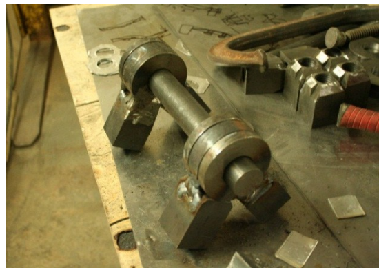
d) Completed Hinges and Shear Pin
