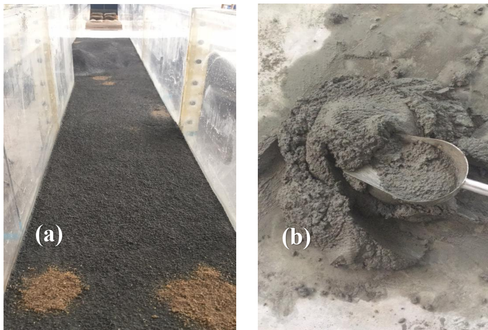
Figure 36. The consolidation process using (a) cement powder and (b) grout.
