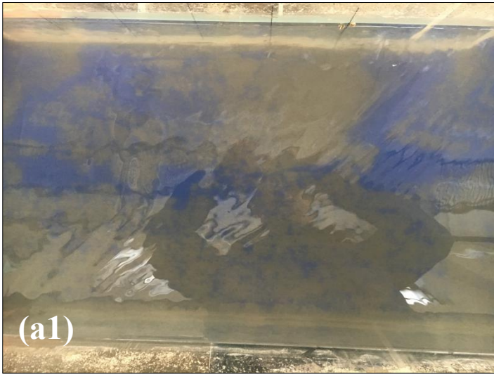
Figure 62. The sedimentation patterns for different feeding locations in case 90_2_3. (a1) (a2) Fed from the left bank of tributary; (b1) (b2) Fed from the right bank of tributary.
