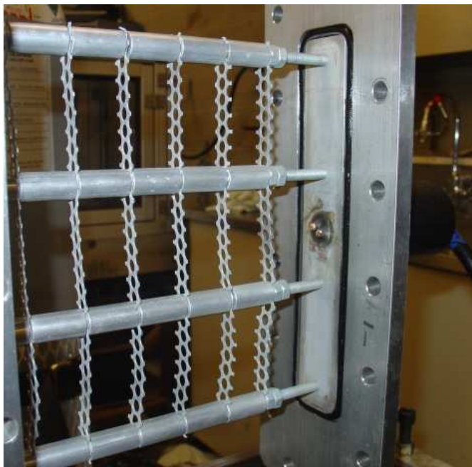
Figure 2.7: A photograph of the wire-mesh used to accelerate the flame generated by the HVI and cause a detonation wave.
