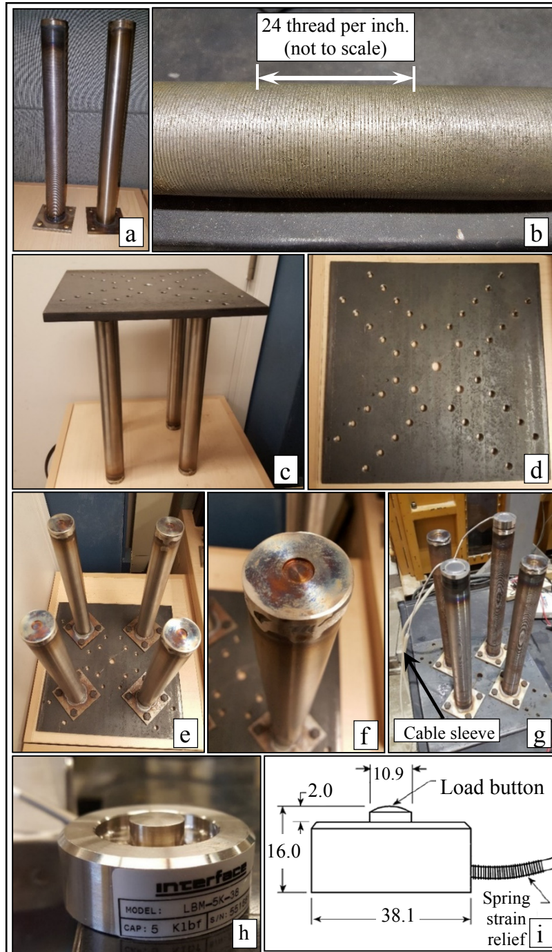
Figure 6.5 Model pile and pile cap; (a) Smooth and rough surface model piles, (b) threading of the rough pile, (c) the full pile group, (d) offset hole pattern on the pile cap, (e) pile tips modification to accommodate the LC1 and LC2, (f) close look at the pile tip modification, (g) LC1 and LC2 at the piles tips, (h) LBM-5K-38 Interface load cell, and (i) schematic diagram illustrate the load cell (all dimensions are in (mm)) (Interface Inc.).
