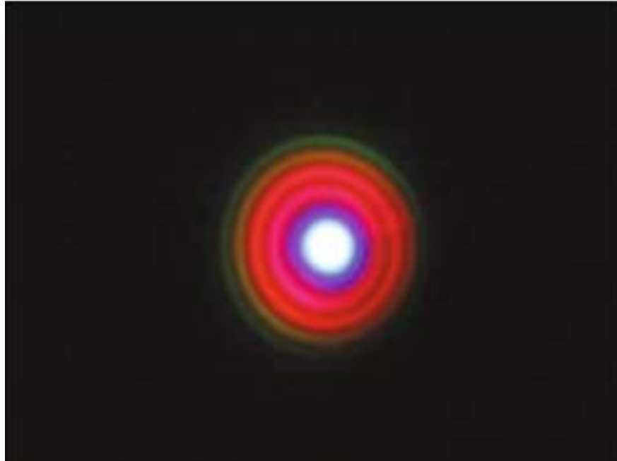
Figure 2.9: Cross sectional image of a filamenting 800 nm, 45 fs, 5 mJ, laser pulse after propagating through 25 m of air. Source: [26]
