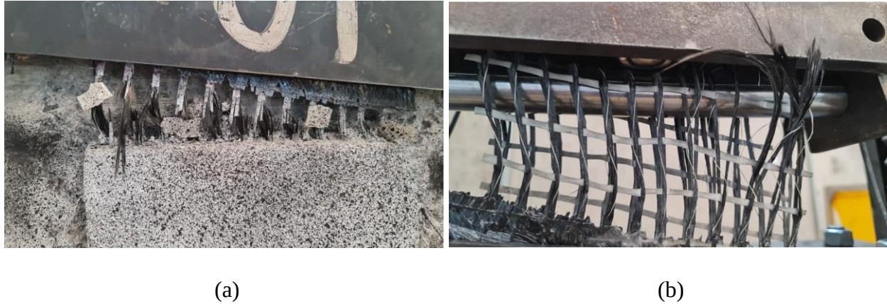
Figure 4.38: fabric rupture near the composite edge (a) and fabric rupture near the grip (b)
