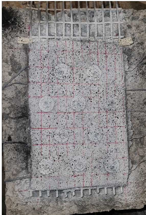
Figure 3.6: Tapes with speckle pattern to track global displacement
