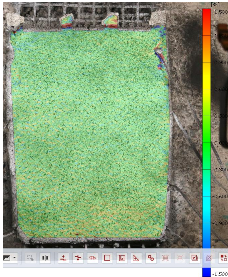
Figure 4.17: DIC generated 2D strain contour map
