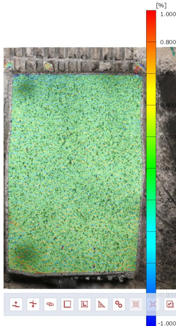
Figure 4.45: DIC generated 2D strain contour map
