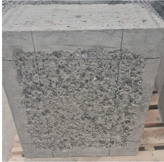
Figure 3.4: Prism surface roughened to a CSP 9
