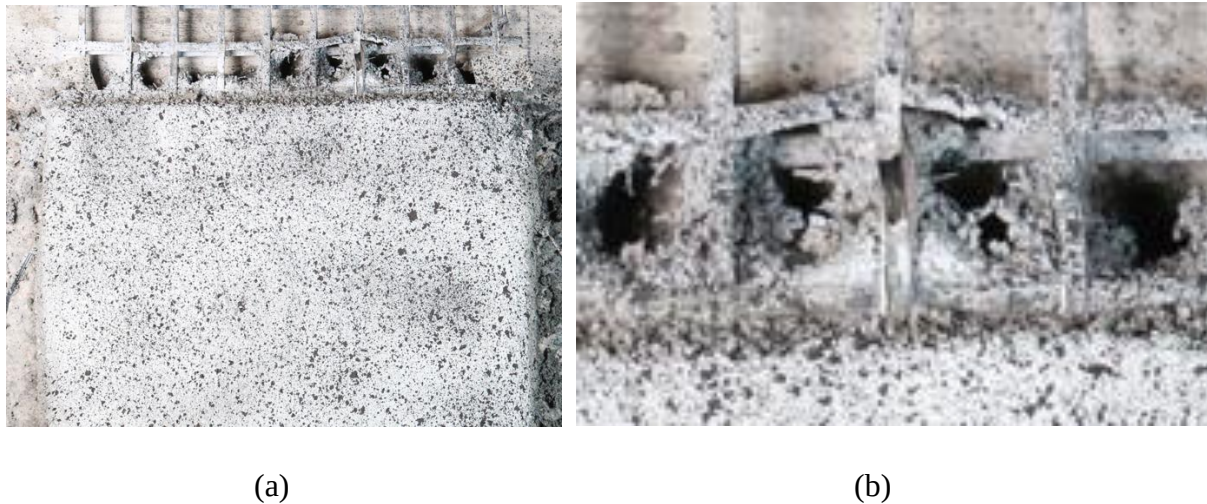
Figure 4.5: front view of the fabric (a) and close-up to the ruptured strands (b)
