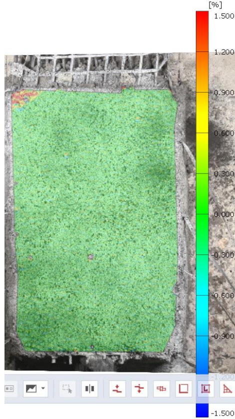
Figure 4.22: DIC generated 2D strain contour map
