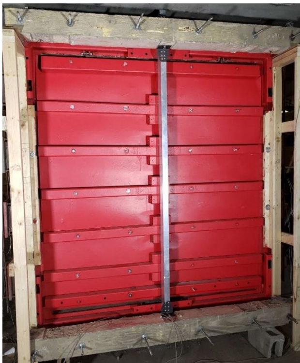
Figure 3.23: M-C2 with brackets at the ends, connected through the mullion end (flange)
