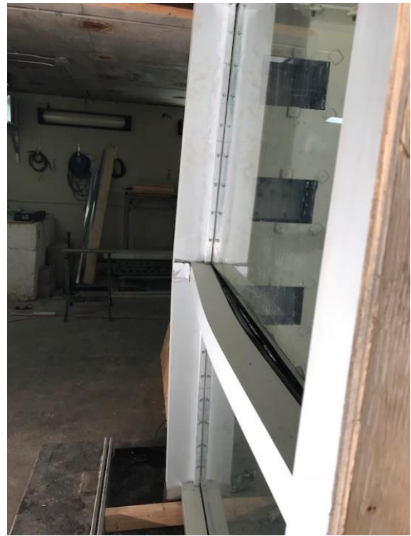
(b) Bending of horizontal mullion
