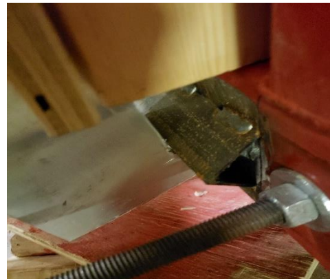
Figure B.4: Failure observation at simple supports
