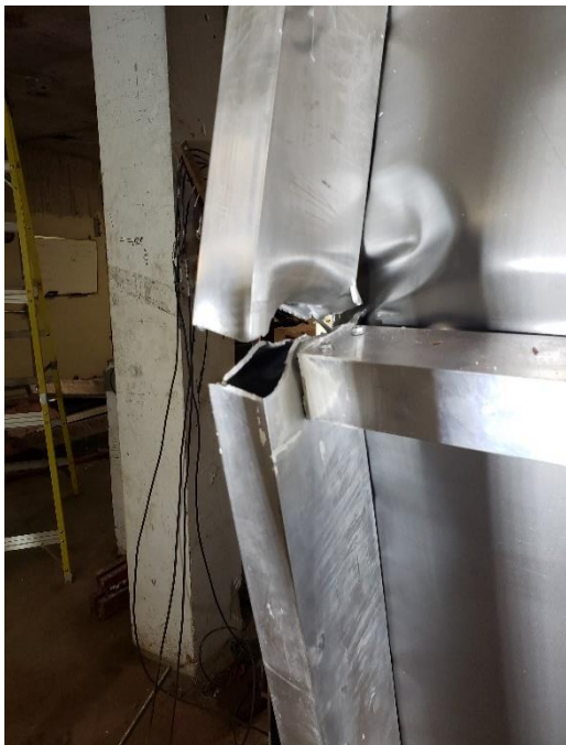
Figure A.3: Close-up failure observation at mid-height of CW1 after testing
