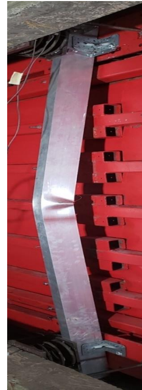
(c) Specimen with damper springs (MC-8) loaded with higher load
