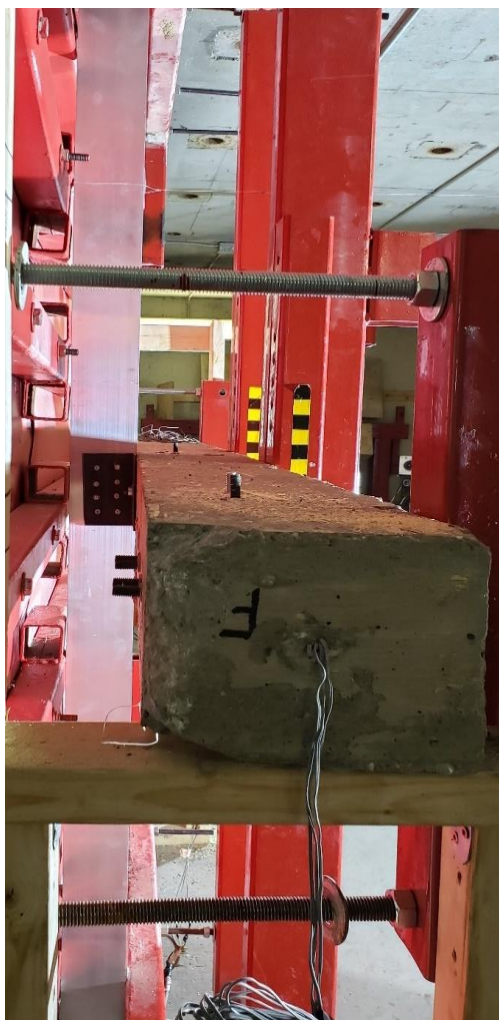
a) Mullion without any damage
