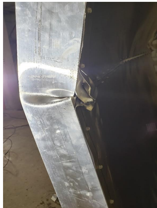
Figure A.3: Close-up failure observation at mid-height of CW1 after testing
