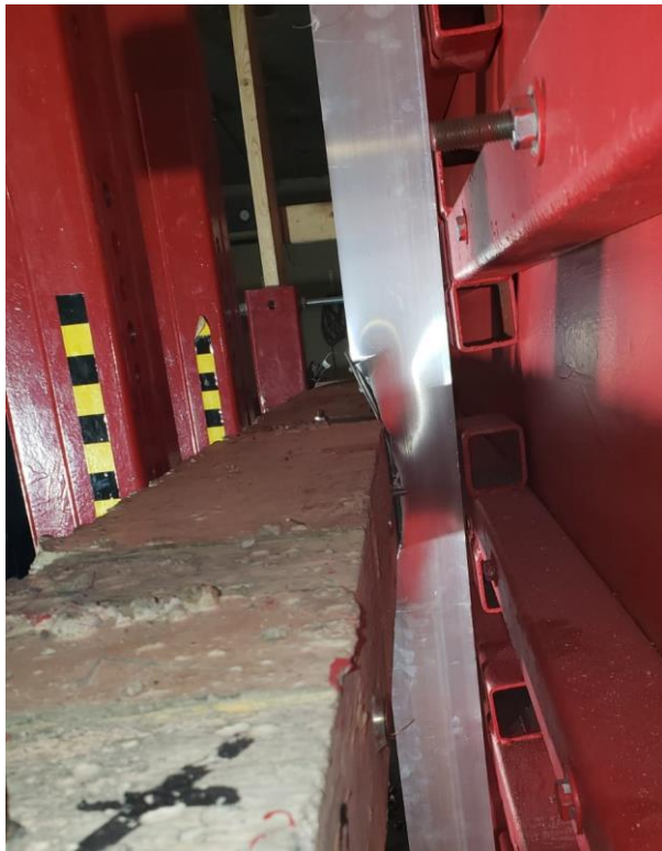
Figure 5.18: Bearing failure of a mullion when bearing against concrete – connection to top and bottom of slab.
