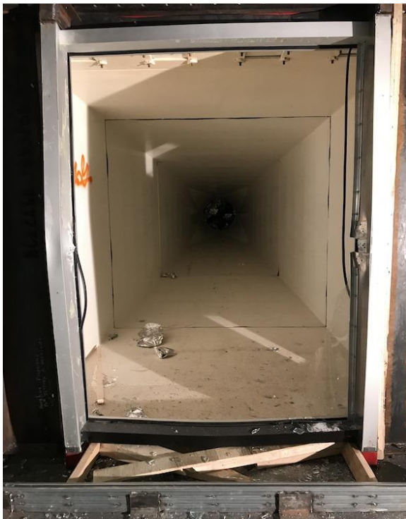
Figure 2.9: Performance of curtain wall during Test 4 (none of the glass panes and horizontal components remained attached to the vertical mullions)
