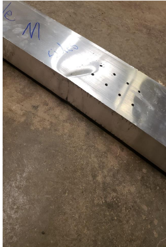
Figure A.13: The mullion deflection and buckling after M-C4 test
