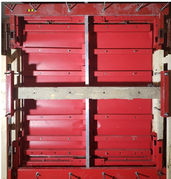
Figure 3.25: M-C4 continuous over the concrete slab, connected on the web of the mullion
