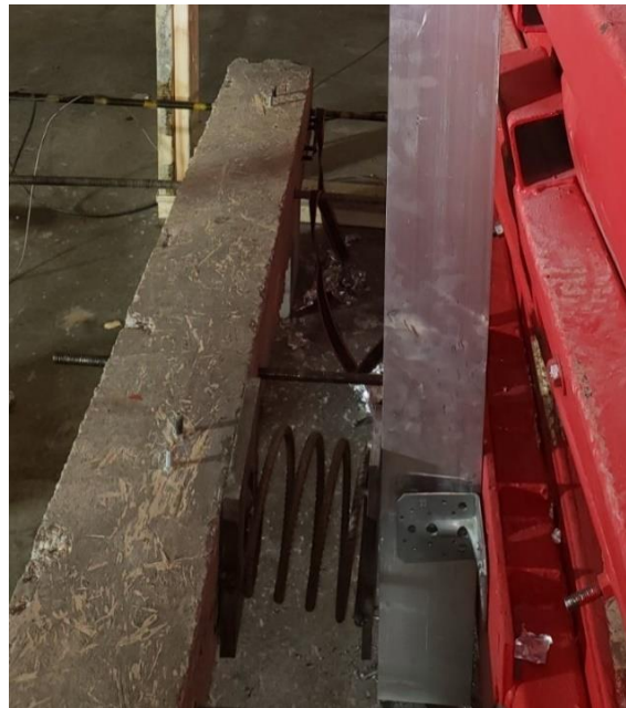
c) Stiffness: 8 N/mm; net length: 160mm
