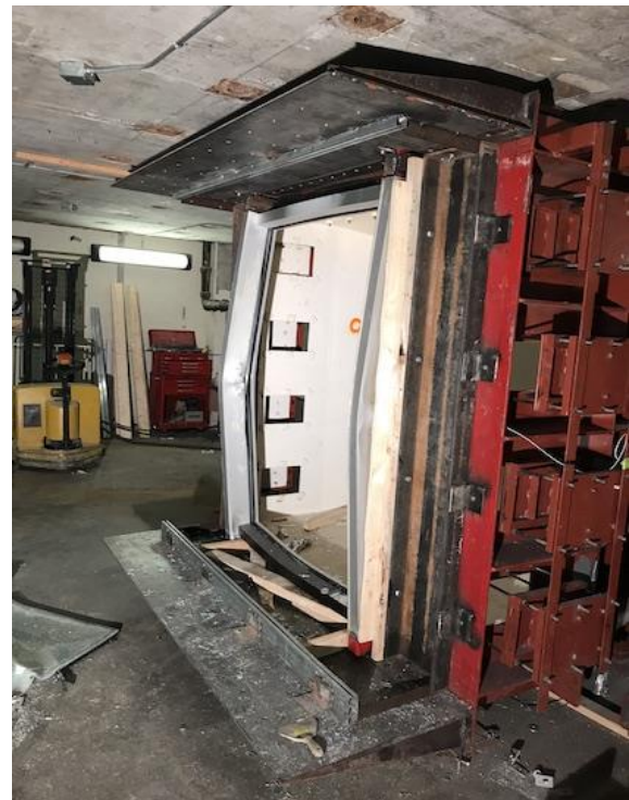
Figure 2.9: Performance of curtain wall during Test 4 (none of the glass panes and horizontal components remained attached to the vertical mullions)
