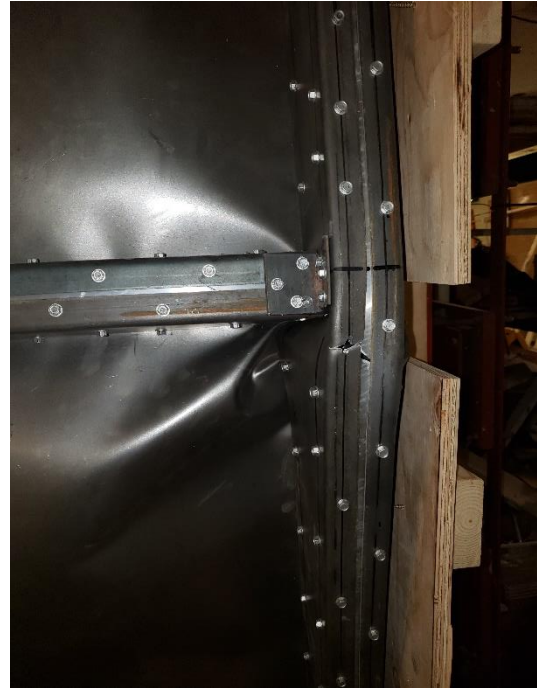
b) Local tension Buckling
