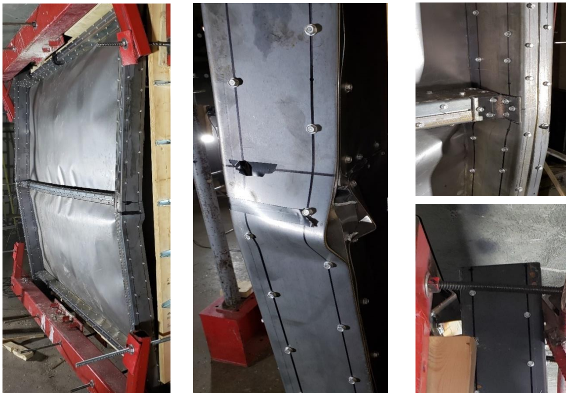
Figure 3.15: Third curtain wall 1st shot; after blast test
