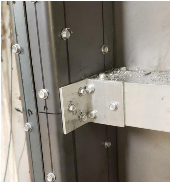
Figure 3.7: Second specimen with retrofitted mullions and anchored aluminum brackets
