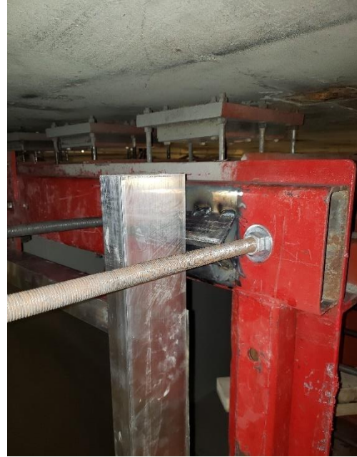
a) Knife-edge support welded on HSS sections
