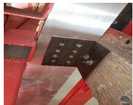
Figure 3.25: M-C4 continuous over the concrete slab, connected on the web of the mullion
