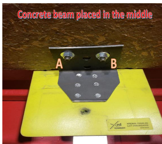
a) Strain gauge locations
