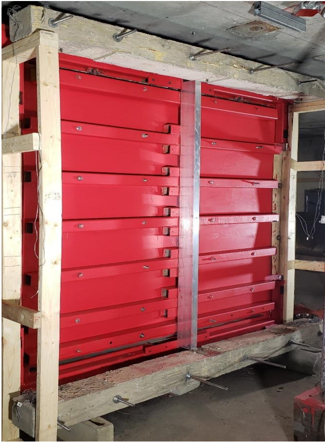
Figure 3.22: M-C1 with brackets at the ends, connected through the mullion sides (web)
