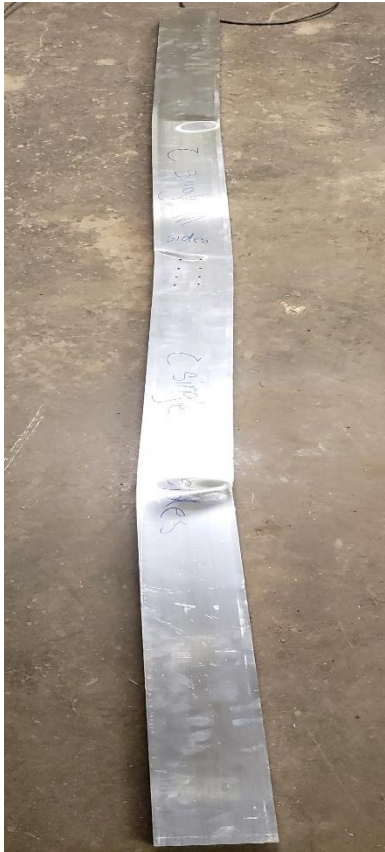
Figure A.13: The mullion deflection and buckling after M-C4 test
