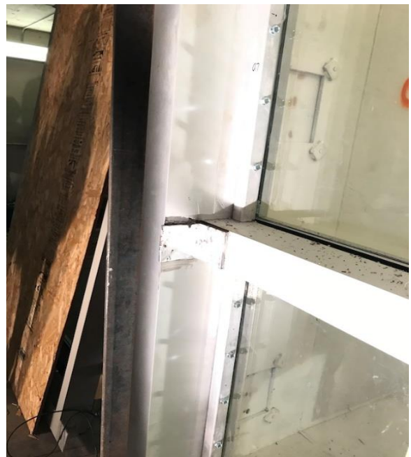
(b) Strengthening mullion connection
