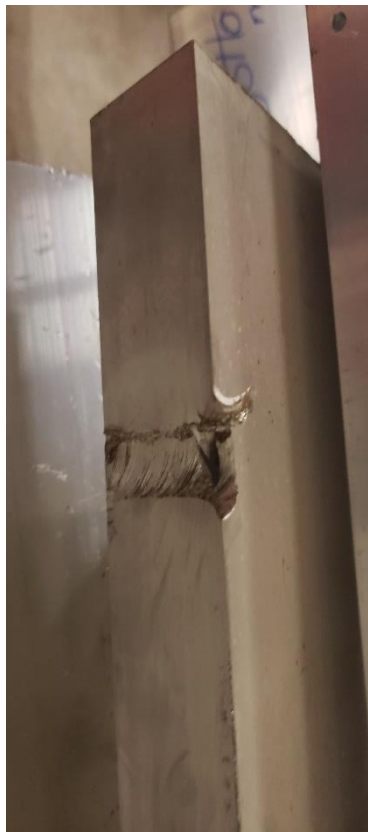
b) Failure at simple support
