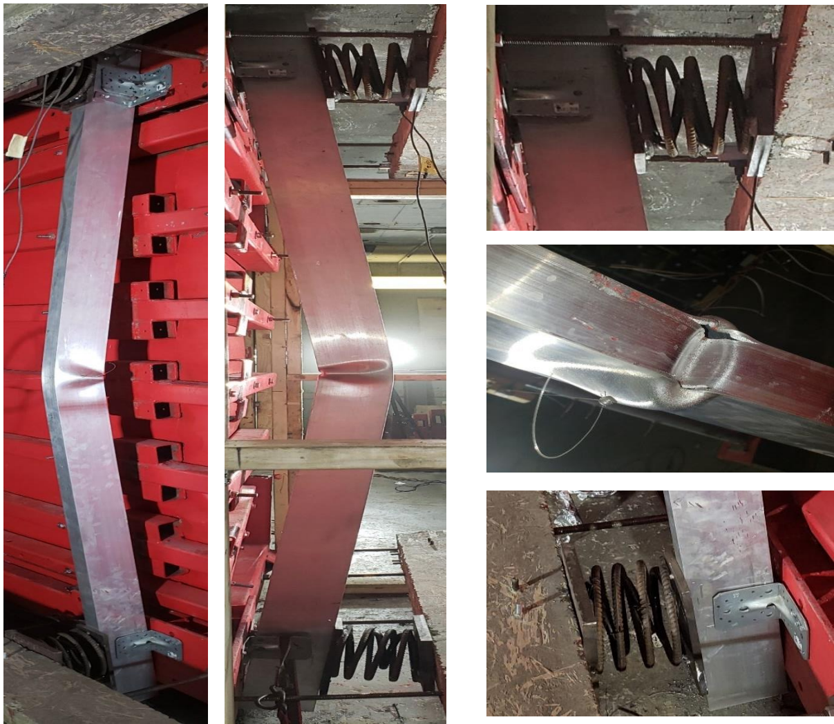
Figure 3.48: Mullion M-C8 after blast shot (single mullion configuration + spring 8 N/mm)
