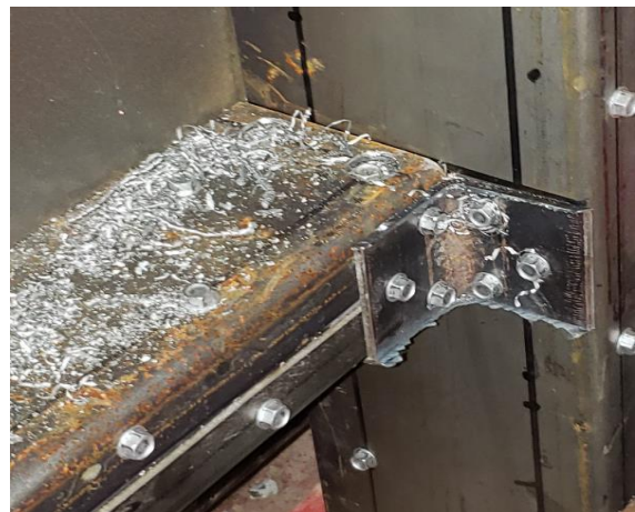
Figure 3.8: Third specimen with retrofitted mullions and transoms, as well as strengthened connections by anchored steel brackets
