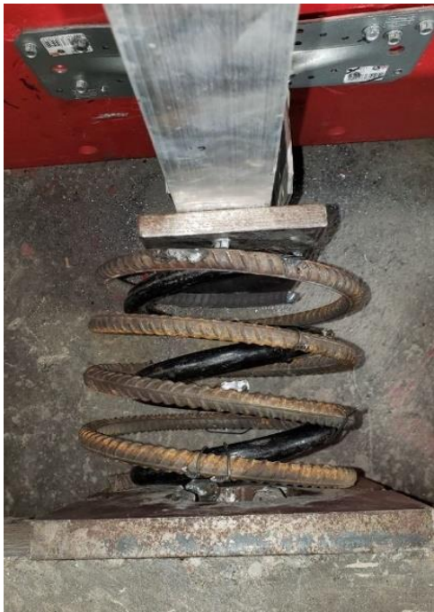
b) M-C8 Stiffness: 30 N/mm Net length: 160 mm
