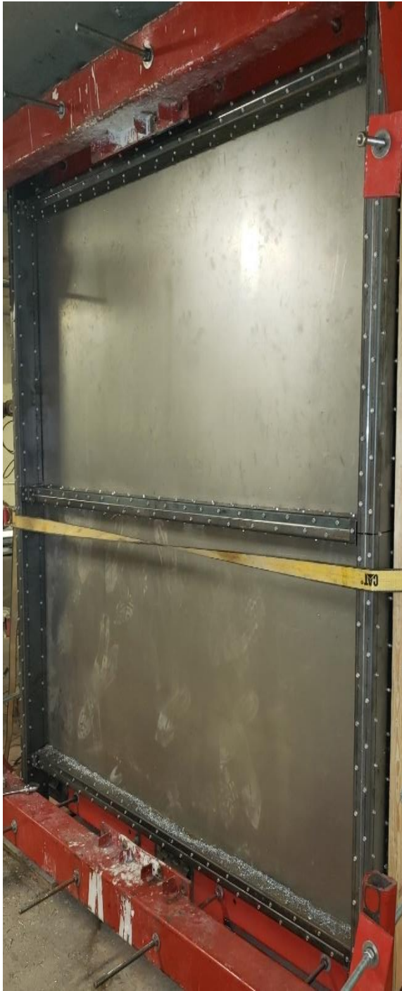
Figure 3.8: Third specimen with retrofitted mullions and transoms, as well as strengthened connections by anchored steel brackets
