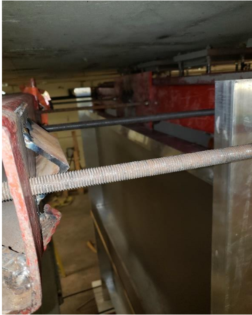
a) Knife-edge support welded on HSS sections
