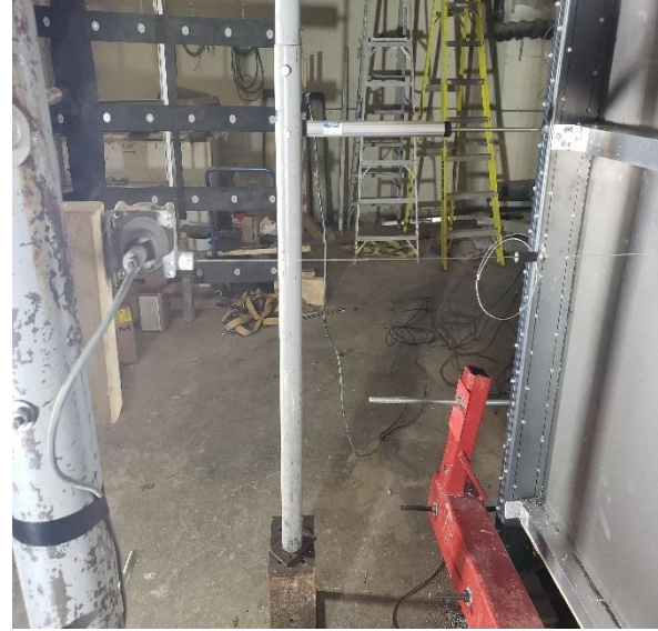
a) Full size curtain wall with two LVDT
