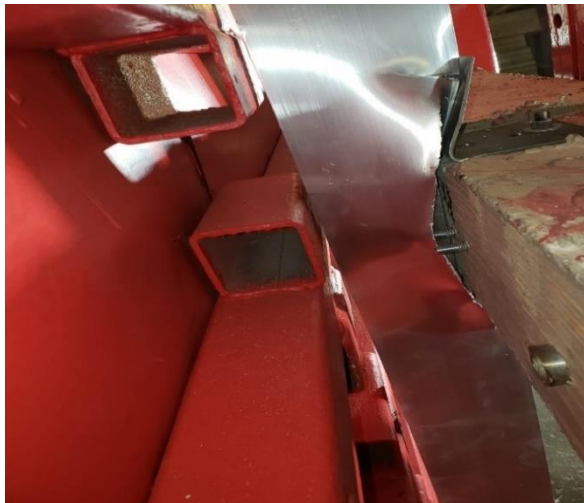
b) Close-up view of mullion failure zone at the middle concrete beam
