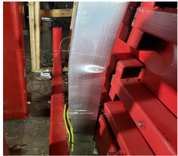
a) Compression buckling at upper and lower sections
