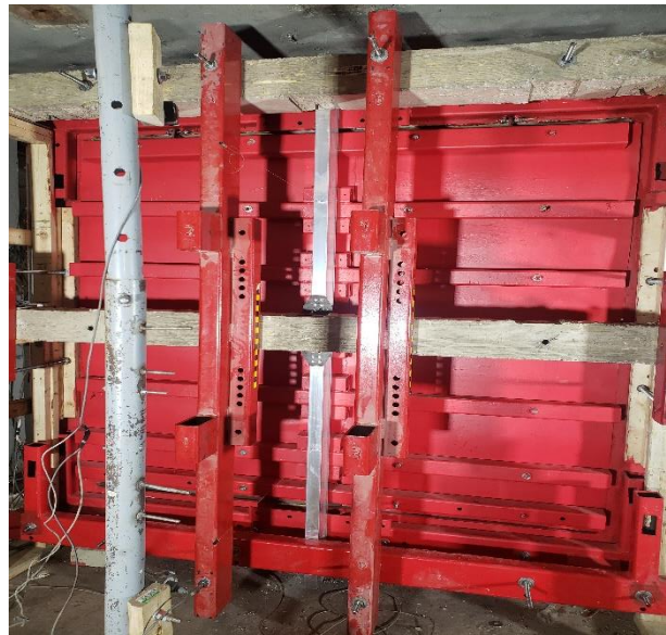
c) Continuous mullion setup with two LVDT
