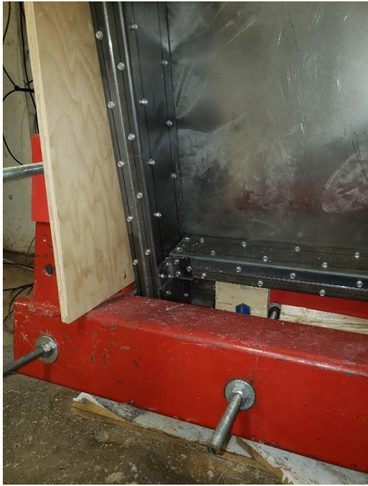
a) In tack anchored steel side brackets
