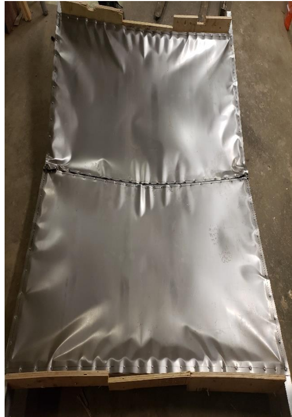
Figure A.2: Steel sheet deformation with no rivet failure after CW1 test
