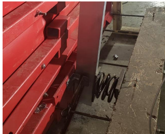
c) support rotation at springs
