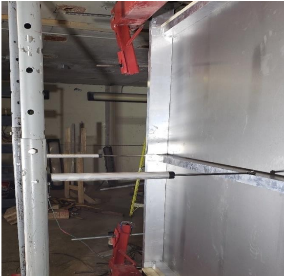
a) Full size curtain wall with two LVDT
