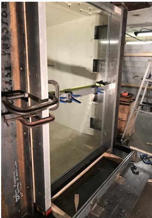
Figure 2.7: Application of aluminum plates and angles with epoxy adhesive for strength enhancement
