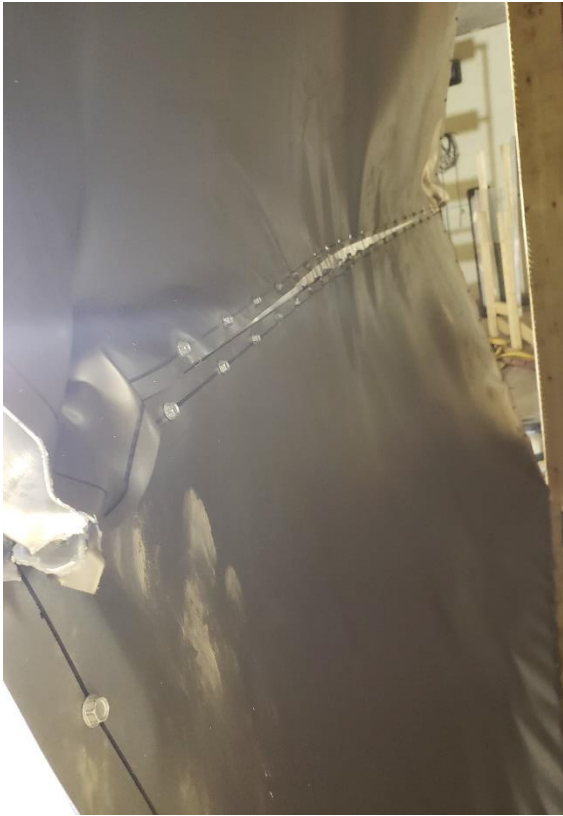
Figure A.2: Steel sheet deformation with no rivet failure after CW1 test
