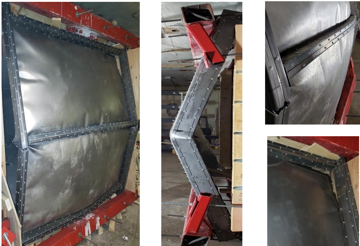
Figure 3.19: Third curtain wall 3rd shot; after blast test
