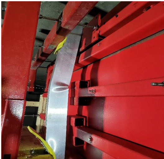
a) Compression buckling at upper and lower sections
