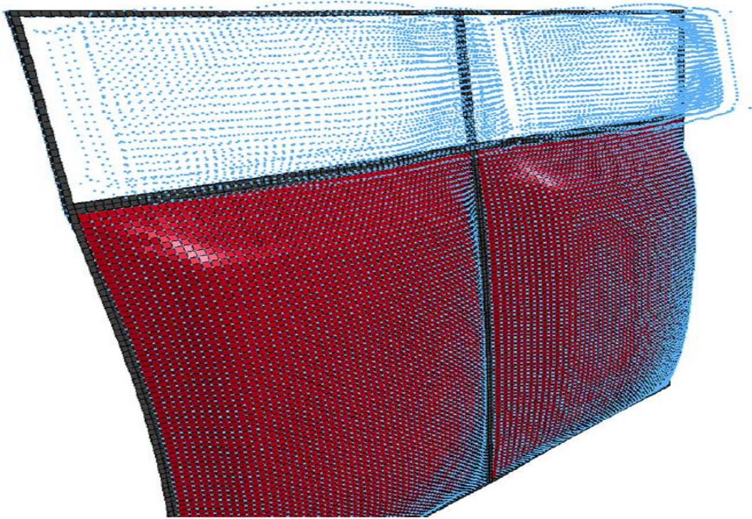
Figure 2.20: FEA representation of glass-break methodology (Kirk et al. 2016)
