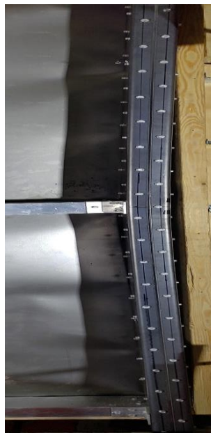
b) Membrane action and its effect on mullions
