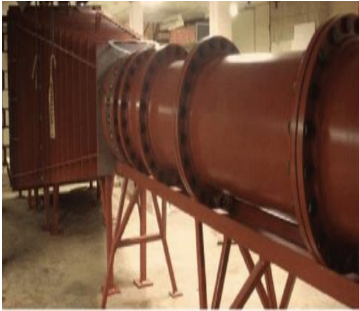
Figure 3.1: Shock-tube assembly; driver section and frame of test area
