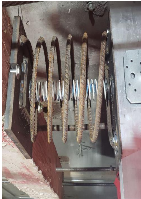
c) M-C9 Stiffness: 23 N/mm Net length: 200 mm
