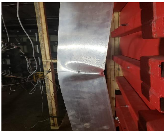
b) Close-up view of mullion failure zone at mid-height
