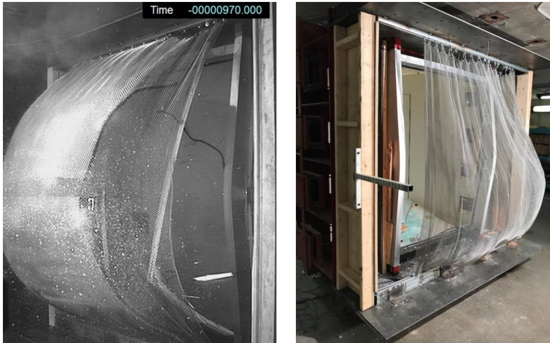
Figure 2.2: Behaviour of the curtain wall during the first test
