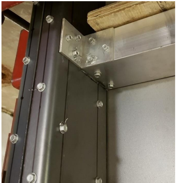
Figure 3.7: Second specimen with retrofitted mullions and anchored aluminum brackets
