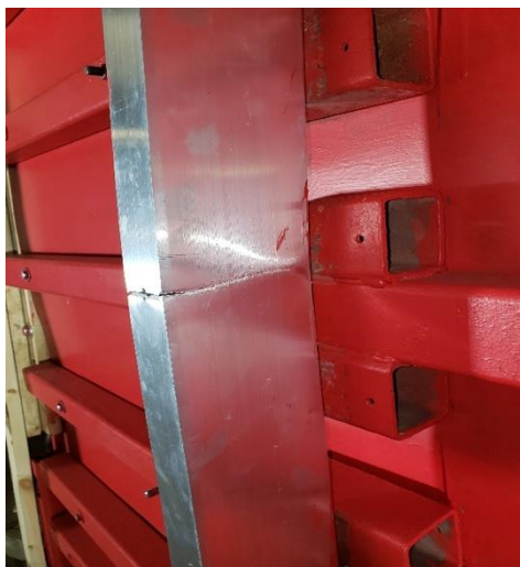
b) Close-up view of mullion deflection at mid-height of single mullion
