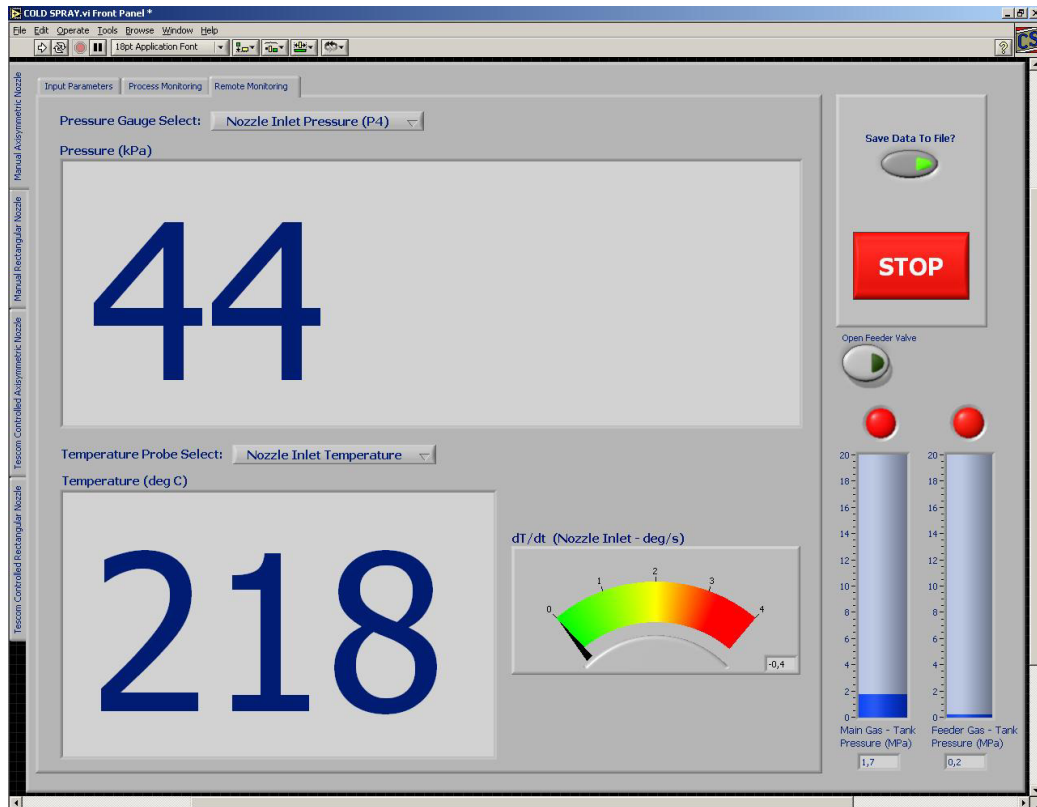
Figure 4.12: Screen capture of the display software used by the operator
