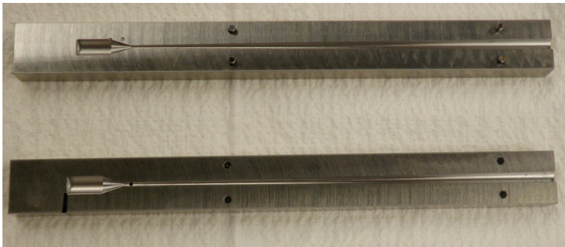
Figure 6.3: View of nozzle sections after manufacturing
