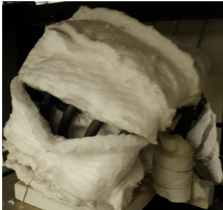
Figure 4.14: Photograph of the insulated driving gas heater
