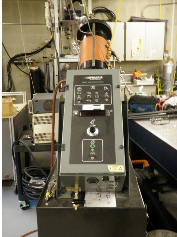
Figure 4.15: Photograph of powder feeder at the University of Ottawa Cold Spray Laboratory
