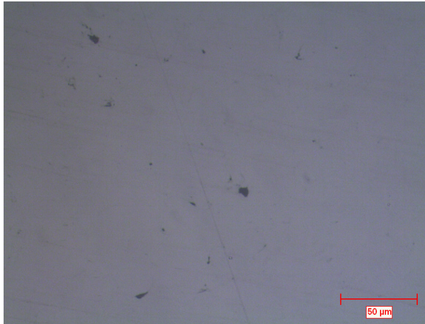
Figure 8.1: View of CGDS CoNiCrAlY cross-section
