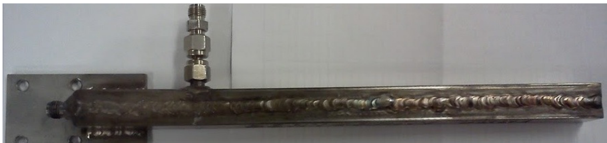
Figure 4.13: View of custom CGDS nozzle.
