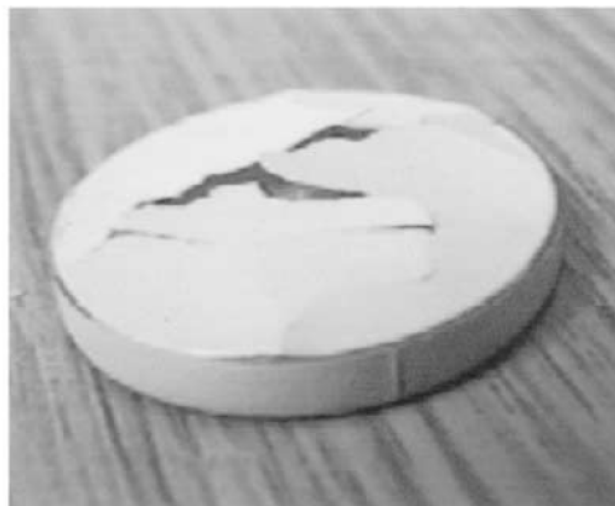
Figure 2.33: Example of a spalled TBC coating during thermal cycling [114].
