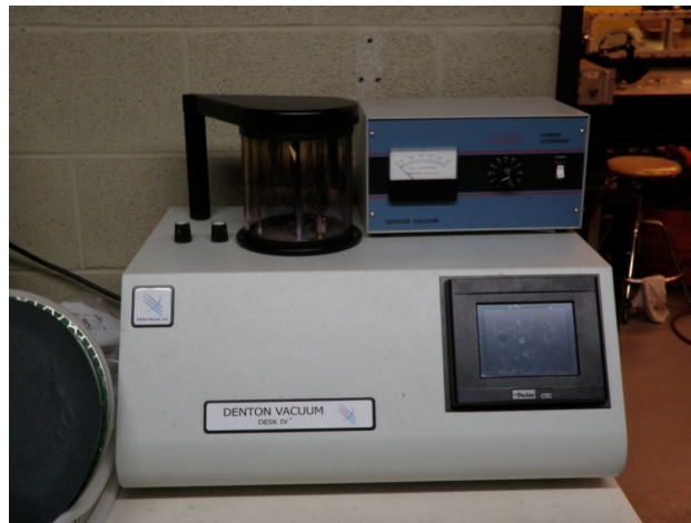
Figure 4.21: Photograph of gold sputter (Denton Vacuum Desk IV)
