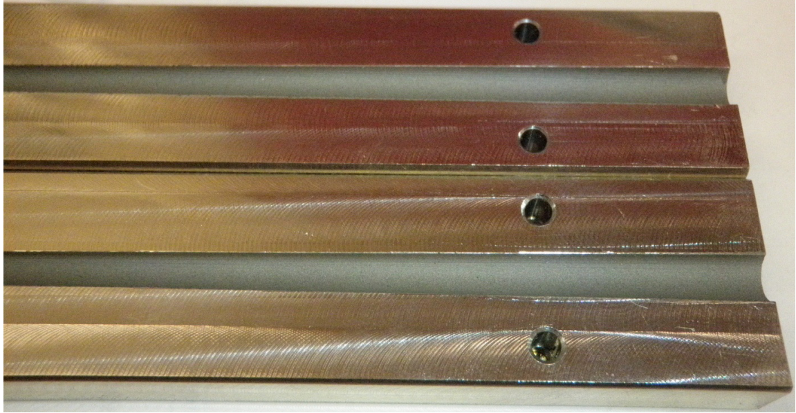
Figure 6.20: Detailed view of coated nozzle: nozzle exit
