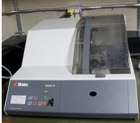
Figure 4.16: Photograph of precision saw (Struers Secotom-10)
