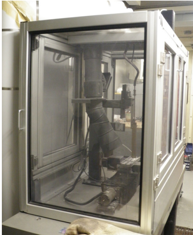
Figure 4.7: Cold spray chamber at the University of Ottawa Cold Spray Laboratory.
