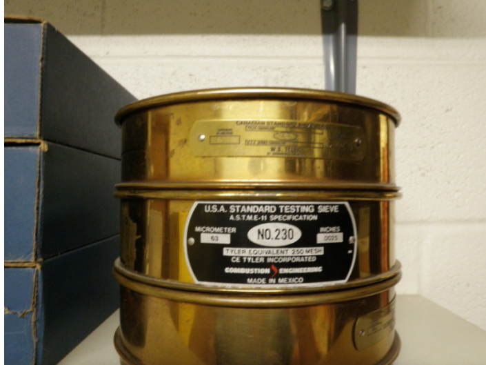
Figure 4.3: Photograph of three stacked sieve drums (CE Tyler)
