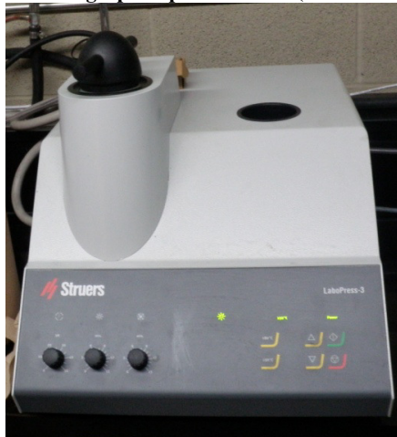
Figure 4.17: Photograph of thermosetting resin mounting chamber (Struers LaboPress-3)
