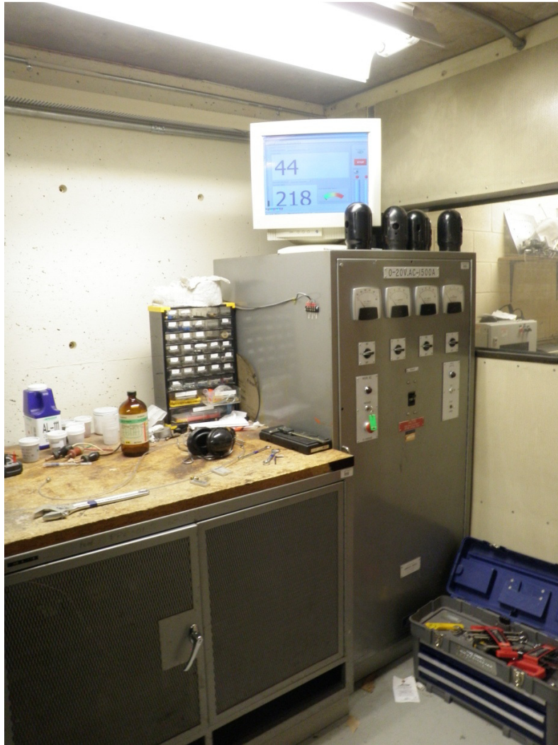
Figure 4.11: View of the CRT display from the operator viewpoint and 30kW power supply
