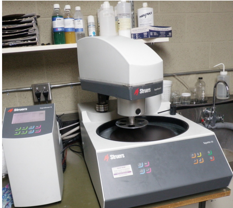
Figure 4.18: Photograph of sample polisher (Struers TegraPol, TegraForce-5 and TegraDoser-5)
