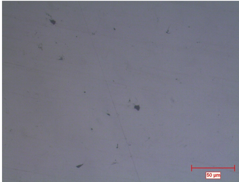
Figure 6.7: View of CoNiCrAlY coating deposited by CGDS
