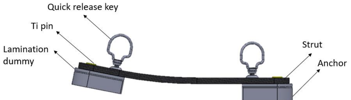
Figure 7-4 Assembly of QRM, dummy plates and strut
