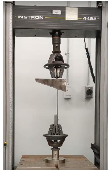
Figure 5-2 Testing setup for downhill walking test
