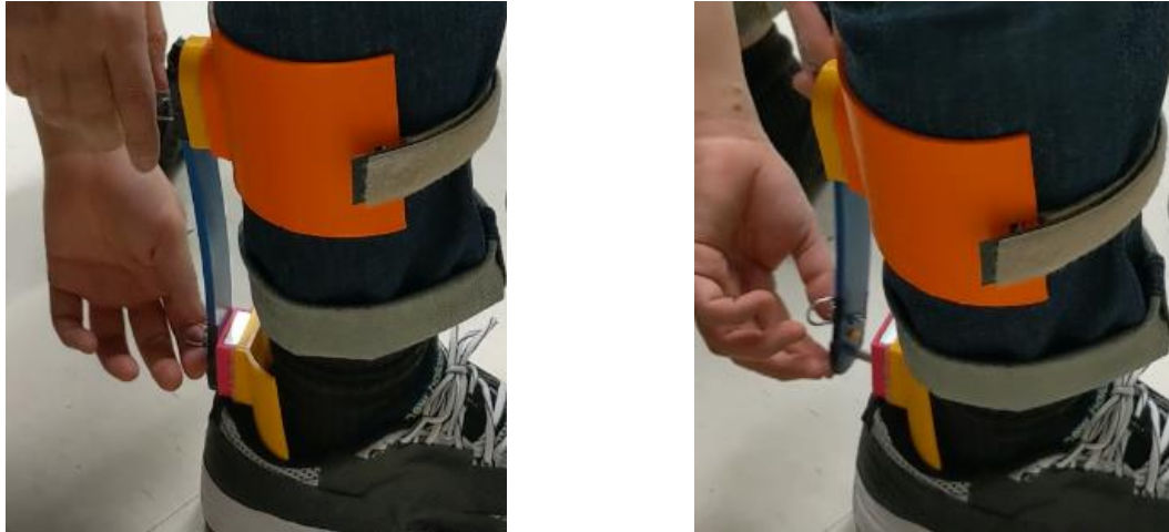
Figure 6-3 An example of the starting of strut removing (left) and starting strut attaching (right)
