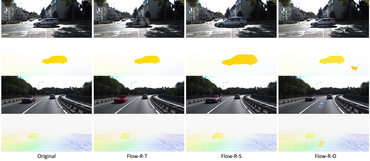
Figure 6.1: Samples of Flow-R. Original and modified images (Row 1 and 3), ground truth optical flows (Row 2 and 4) are shown. The first column displays the original data from the KITTI dataset. The second column shows the data with the texture of the main object of car replaced. The third column shows the data with the shape of the main object rescaled. The fourth row presents the data with an unseen object added.
