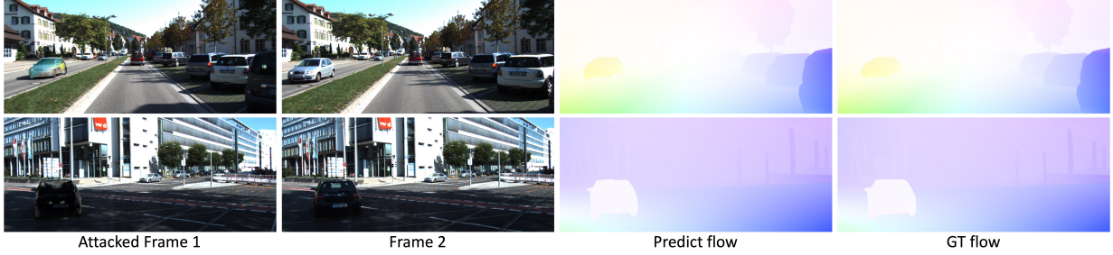
Figure 6.3: Texture Attack. The texture of the main object (car) in the first frame is replaced, while the second frame remains unchanged. The resulting optical flow is similar to that derived from the original images.
