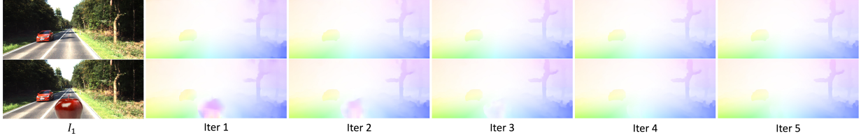
Figure 6.10: Visualization of Intermediate Flows in the Decoder. Decoder GRU iterations in original and failed samples.
