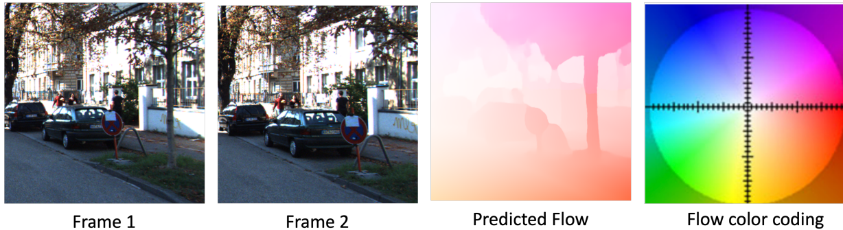
Figure 2.1: Visualization of dense optical flow in KITTI [34] dataset.
