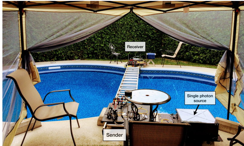
Fig. 5. Image of outdoor underwater link in an in-ground swimming pool. The single photon source, on the sender's side, is enclosed within a black box. The sender's setup is mounted on an optical breadboard and consists of a microscope objective stage, a spatial light modular, mirrors and a periscope which brings the beam in an air-filled aquarium that is half-way under the water. In order to stabilize the aquariums, they are secured to a ladder that is placed above the underwater link, but is not in direct contact with the optical breadboards. The idler photon is sent from the sender to the receiver through a single mode fiber that is mounted along the ladder. The receiver's setup is mounted on an optical breadboard and also consists of a periscope, mirrors, a spatial light modular and a microscope objective. Red lines were added to outline the beam's path.
