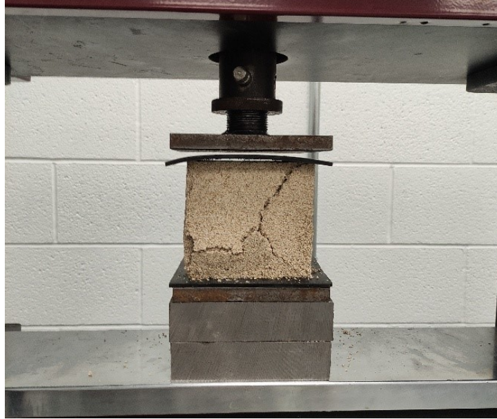
Figure 5.10 Compressive Strength test, HLC cubes after failure.
