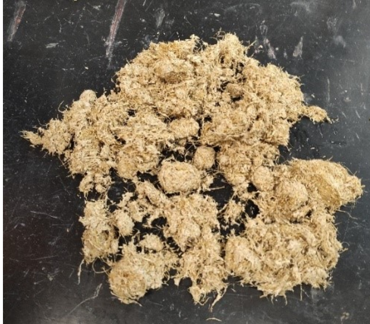
Figure 5.4 Balling effect of hemp fibres.
