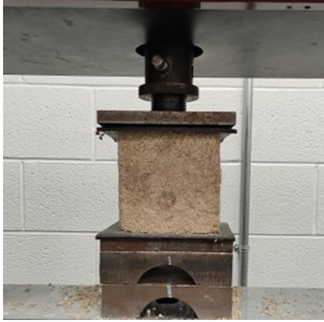
Figure 3.5 Compressive strength testing setup.
