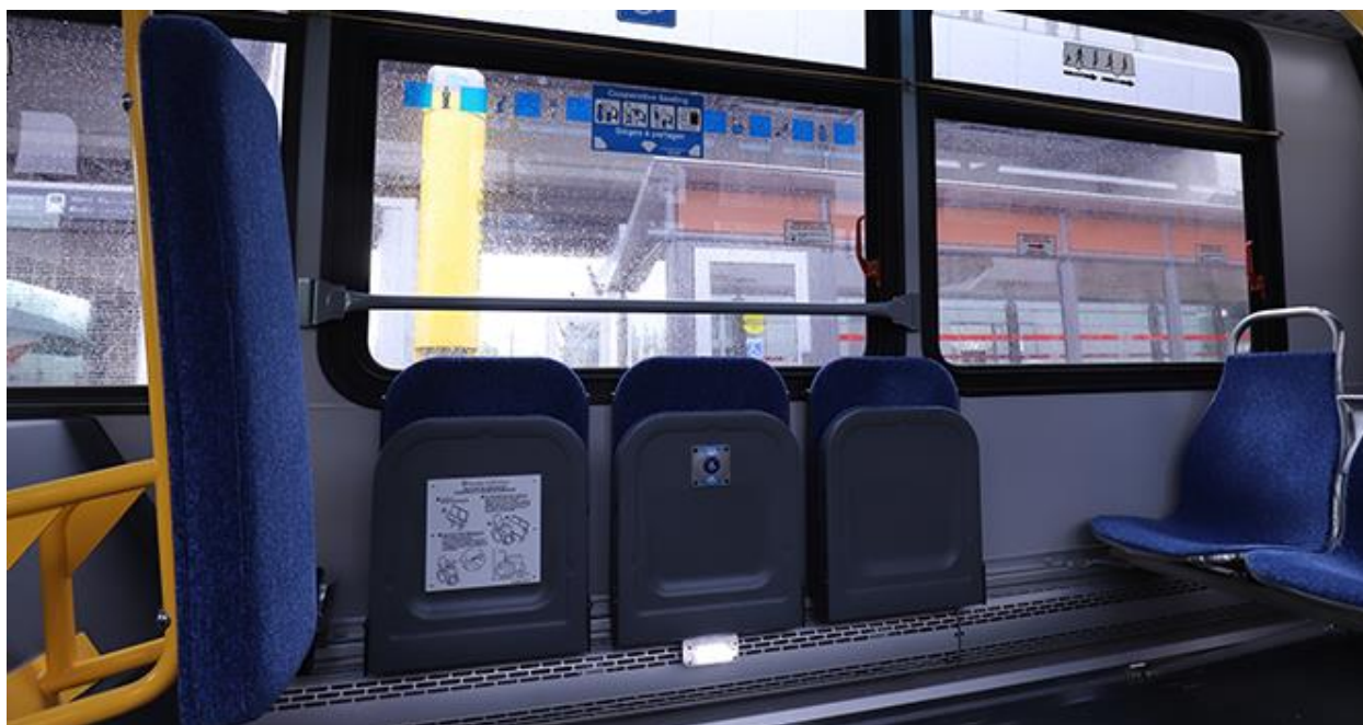
Figure 31: A photograph of the front of the bus intended for passengers using mobility devices, such as strollers and wheelchairs. Credit: OC Transpo
