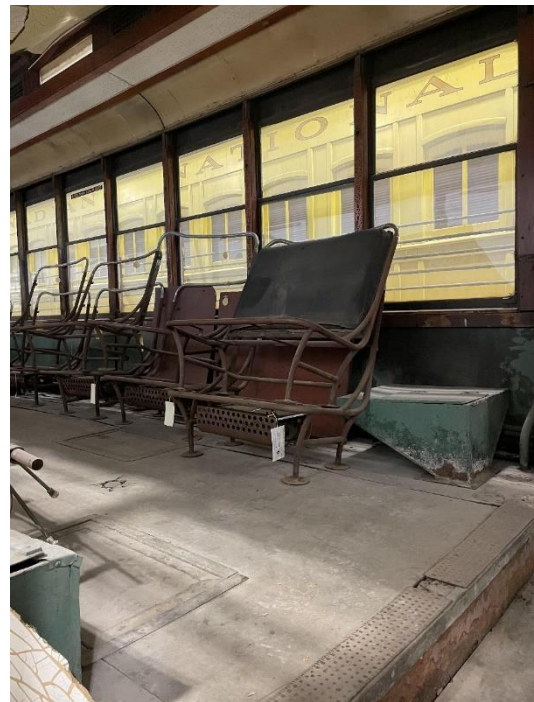
Figure 15: Stacked seats feature the raised grab rail on the backrest. Credit: Ingenium.
