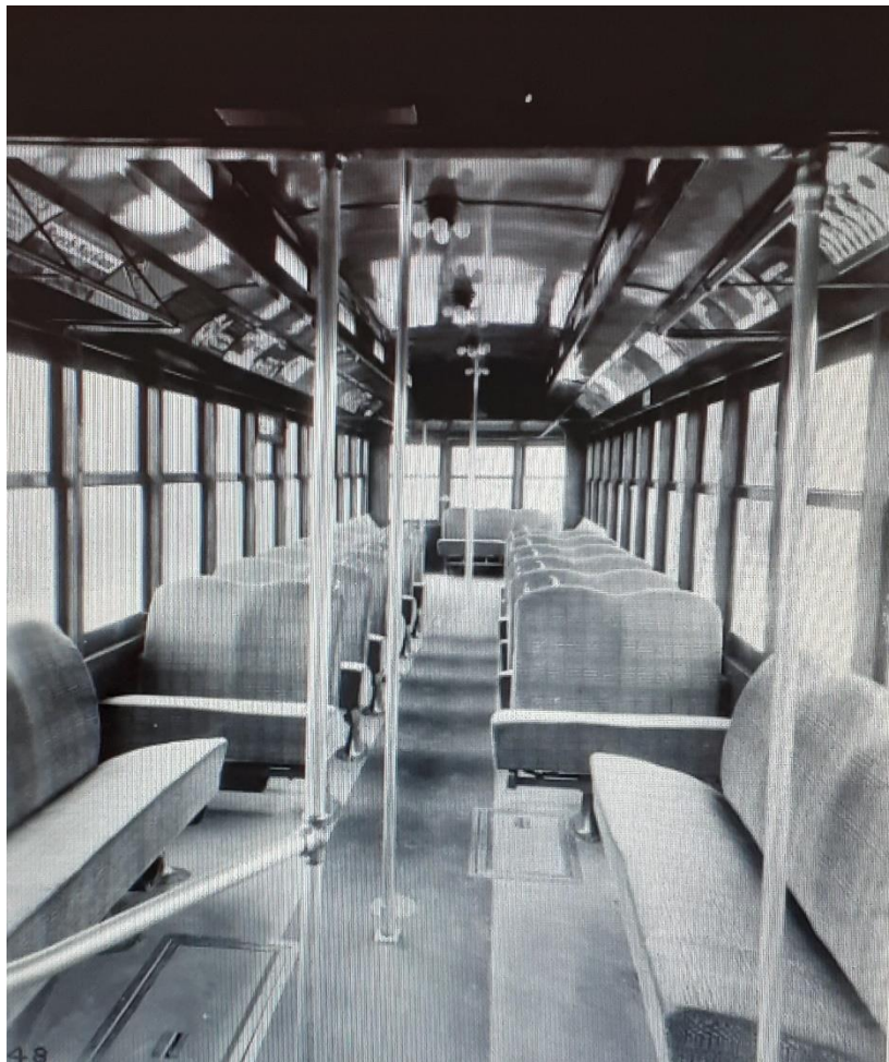
Figure 17: Inward facing benches were introduced by the OER during the Second World War in an effort to encourage passengers to move to the back of the streetcar. Credit: City of Ottawa Archives, CA 1535.
