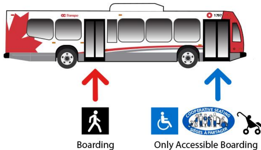
Figure 30: A drawing of a standard low-floor rigid bus operated by OC Transpo, marking the accessible entrance at the front and the step-up entrance on the side. Credit: OC Transpo
