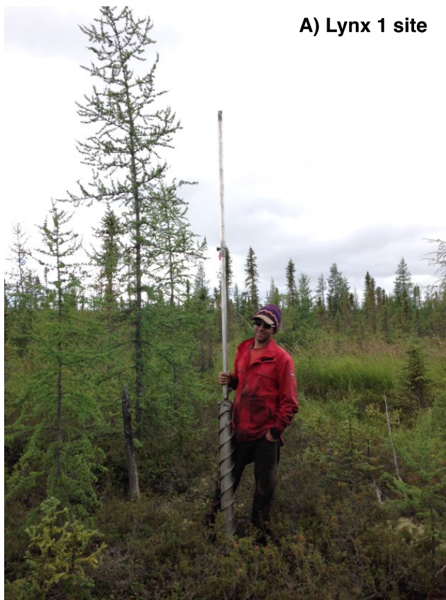
Figure 9 (A) Sampling with a CRREL corer and Viper powerhead at Lynx 1 during summer 2014. (B) Thaw slump headwall sampling in summer 2013 with a handheld HILTI corer at the CB and (C) Wilson sites.
