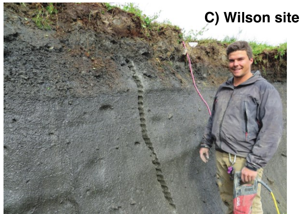
Figure 9 (A) Sampling with a CRREL corer and Viper powerhead at Lynx 1 during summer 2014. (B) Thaw slump headwall sampling in summer 2013 with a handheld HILTI corer at the CB and (C) Wilson sites.
