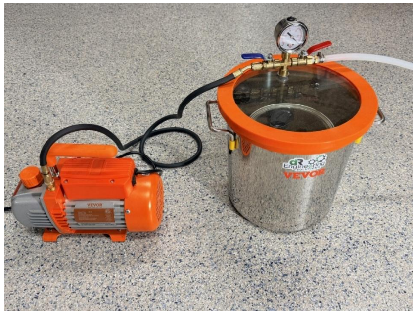
Figure 3.10: Vacuum pump (left) and vacuum pot (right)
