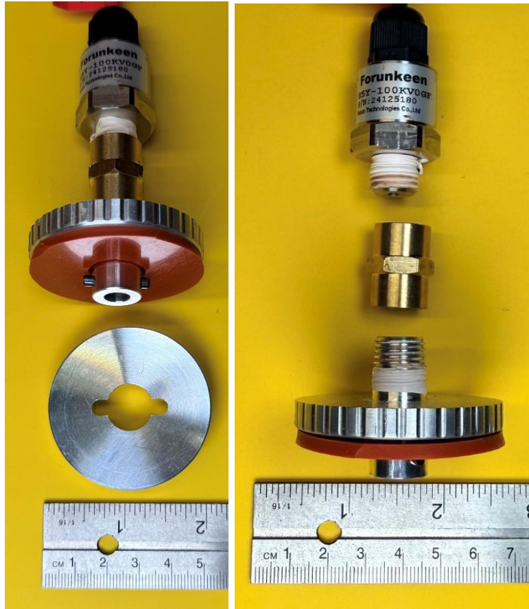
Figure 3.13: PT with vacuum valve assembled (left) and PT disassembled (right) having PT (top), 6mm (1/4" NPT) female pipe coupling (middle), vacuum film connector plates (bottom)
