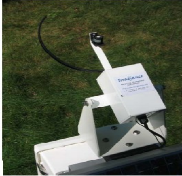
Figure 2-10 Rotating shadowband manufactured by Irradiance Inc. This measures GHI, DHI , and calculates DNI [29].
