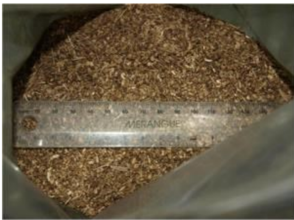
(A) Fines: Material passing through a 3.18 mm (1/8") sieve screen
