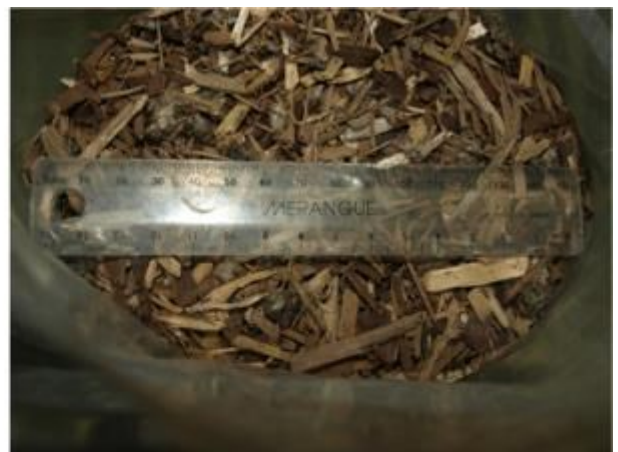
(B) Mids: Material retained between 3.18 and 6.35 mm (1/8" and 1/4") sieve screens
