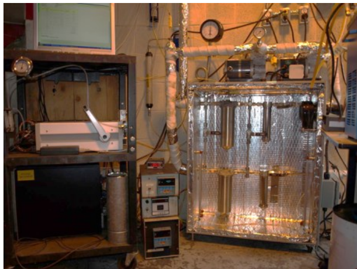
Figure E.1: Gas sampling system in the small pilot scale gasification laboratory (open heated filter cabinet, heated head sampling pumps and micro-GC are visible)
