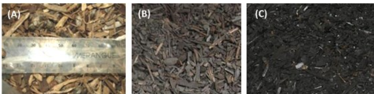
Figure 4.1: Photographic comparison of (A) parent material, (B) torrefied material, and (C) carbonized material.
