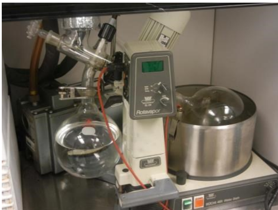
Figure E.4: One of the rotary evaporators used to determine the amount of gravimetric tar
