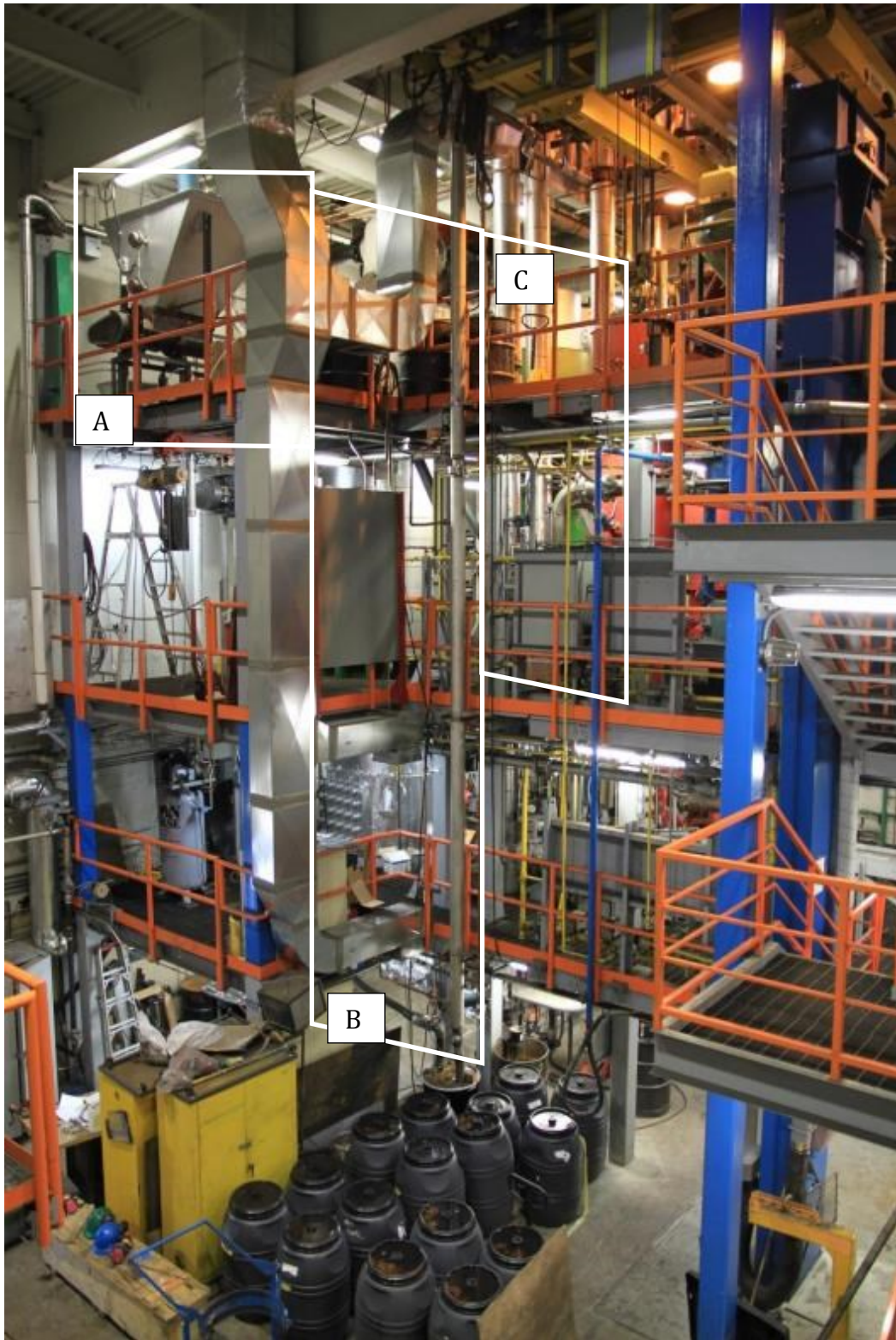
Figure 5.4: Picture of the BFB laboratory. (A) Indoor feed bin, (B) location of the reactor and (C) Location of the cyclone.
