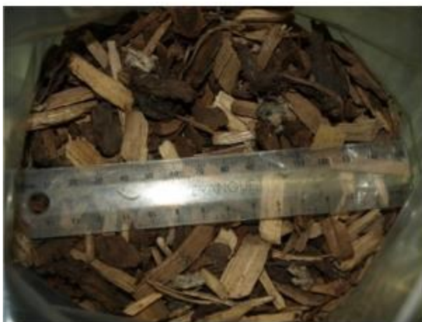
(C) Coarse: Material retained between 6.35 and 19.05 mm (1/4" and 3/4") sieve screens
