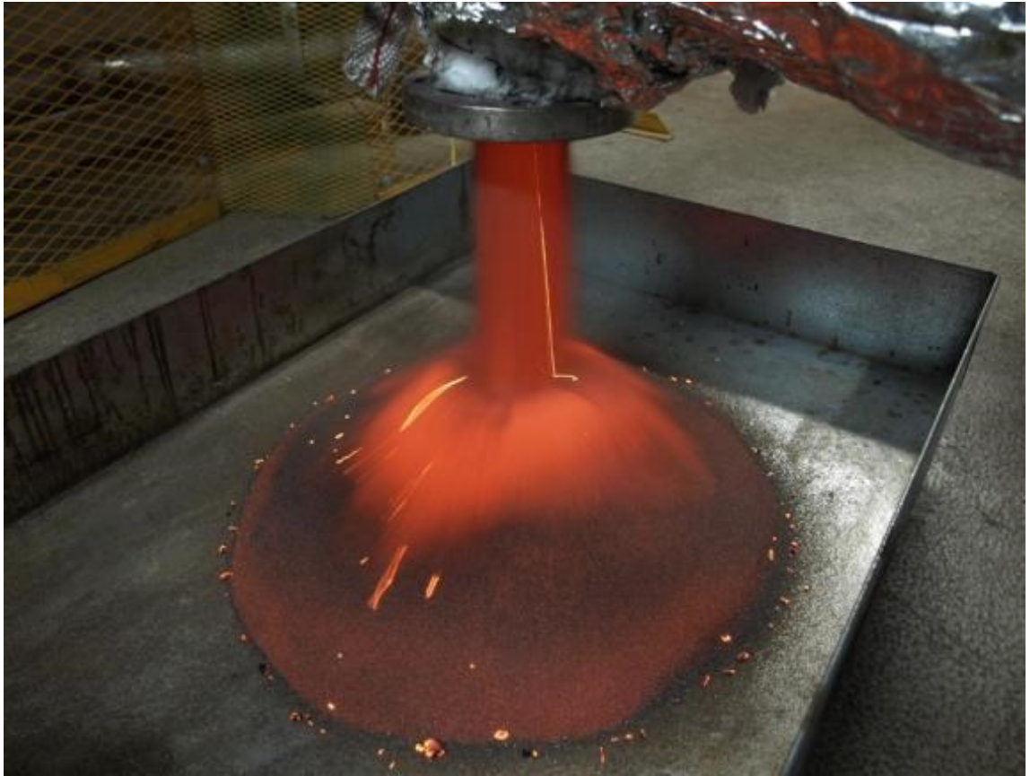
Figure E.5: Bed material samples taken during operation of the large pilot-scale gasifier
