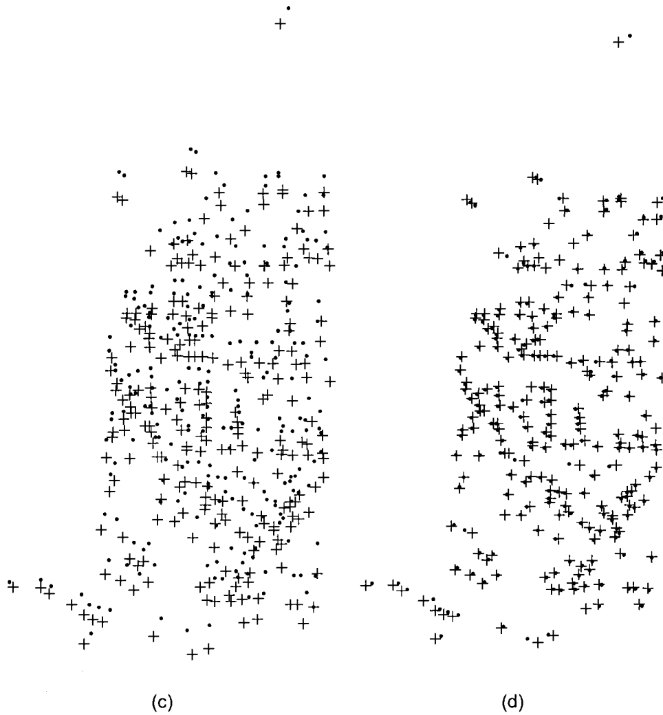
Figure 3.4 Results for experiment 1 (continued). (c) The relationships between matching features after registration using the traditional approach. (d) The relationships between matching features after registration using the proposed algorithm.
