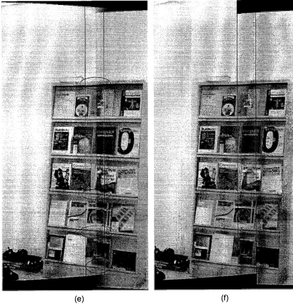
Figure 3.4 Results for experiment 1 (continued). (e) Stitching result with traditional registration approach but blending on a strip block. (f) Stitching result after registration using proposed method and blending on a strip block.
