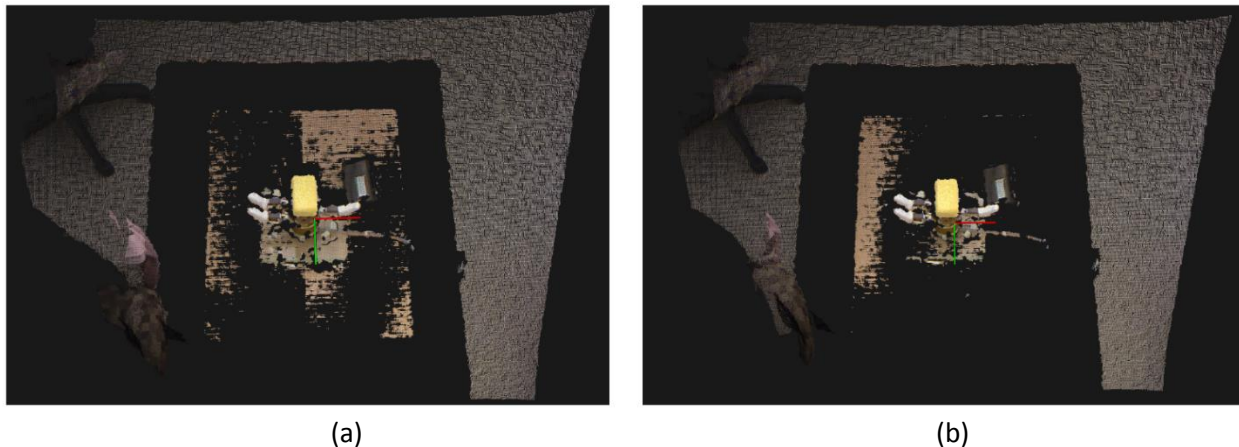
Figure 4.8: (a) Planar background removal with RANSAC parameter t=0.5 cm; and (b) with t=0.75 cm.
