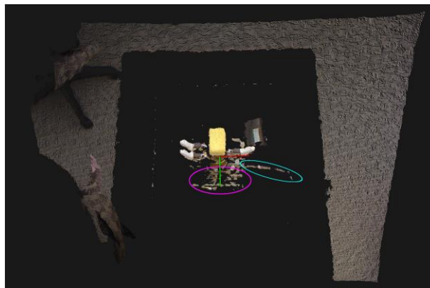
Figure 4.9: Planar background removal with RANSAC parameter t=1 cm.
