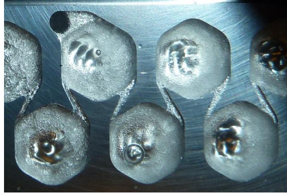
Figure 7.4 Purging prior to mass transfer test in reactor 412S showing dead zones (total flow rate approx. 35 mL/min) in the centre.
