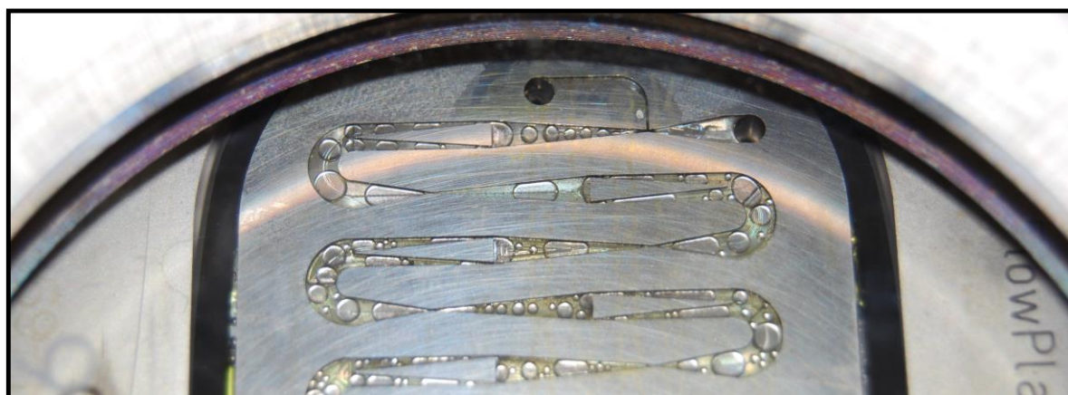
Figure 1.2 Hydrolysis of 4-nitrophenyl acetate in an obstacle based mixing structure
