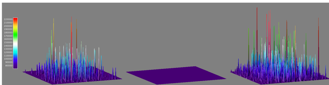
Figure 3-20. 3D accumulated bright events (500 frames) of 15 at 100 pM concentration (left), disappearance of signal after flowing water (middle), and recovery of signal after flowing 100 pM 15 again (right). The area shown corresponds to an 80 \mu\text{m} square.
