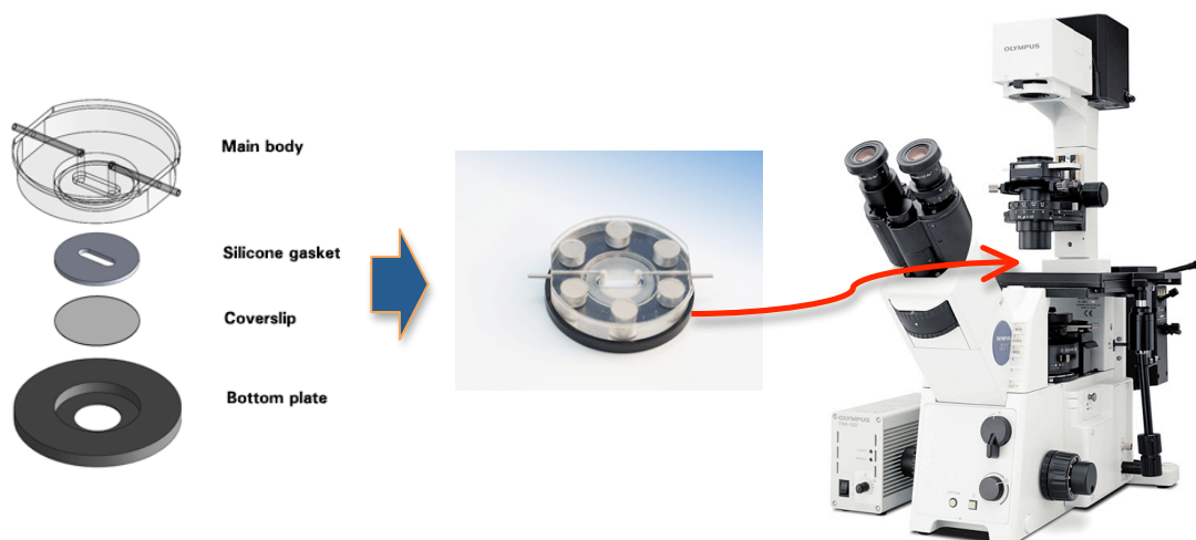
Figure 3-21. Chamlide flowcell reactor design and orientation in TIRF microscope. Images adapted from Chamlide ( www.chamlide.com ) and Olympus Microscopy ( http://www.olympuscanada.com ).
