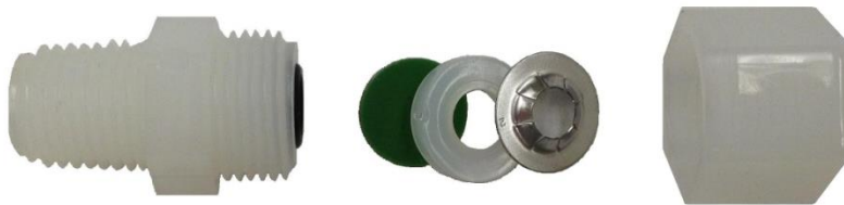
Fig. A.2. PVC fitting and septa for sealing gas sampling ports through the wall of column.
