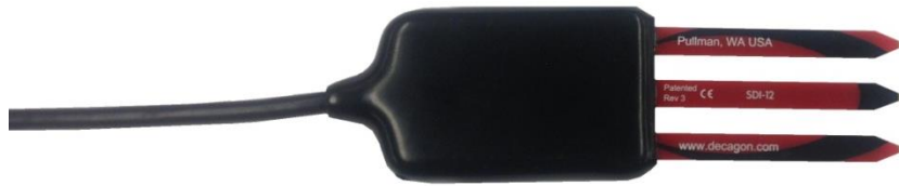
Fig. A.4. 5TM sensor for measurement of VWC.
