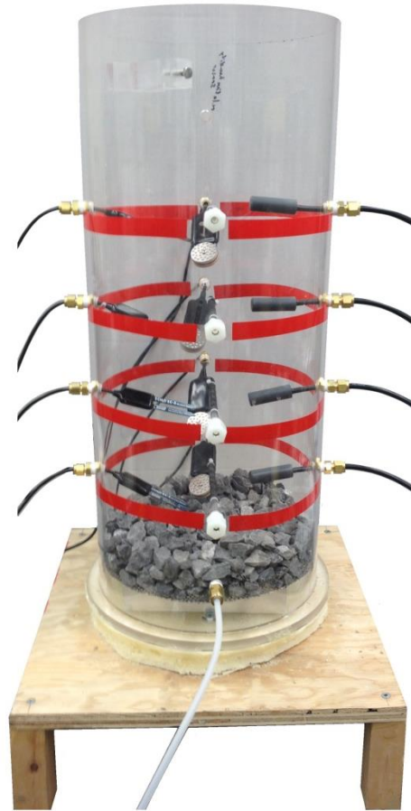
Fig. A.10. Front view of column base, drainage layer, gas distribution layer, sensors, and gas sampling ports.
