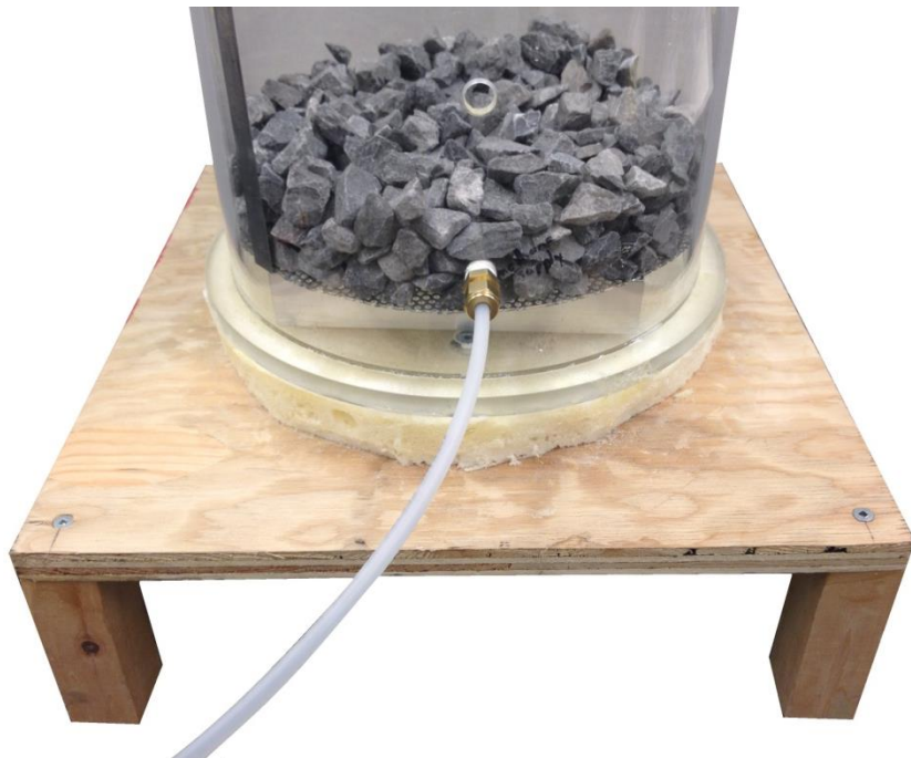
Fig. A.9. Front view of column base, drainage layer, and gas distribution layer.
