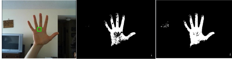
Figure 28 Example Result 1. The left back projection has holes that are fixed in the right back projection
