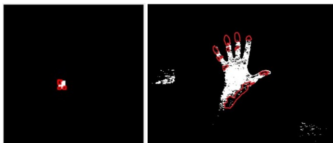
Figure 27 CrCb histogram (left) and corresponding back projection (right).
