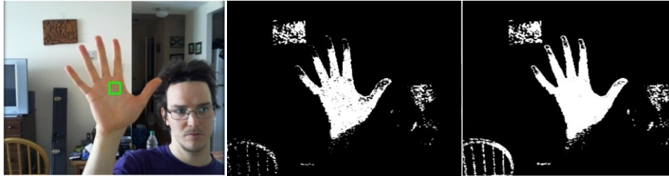
Figure 29 Example Result 2. The left back projection is missing large portions of the fingertips. The fingertips are much better segmented in the right back projection.
