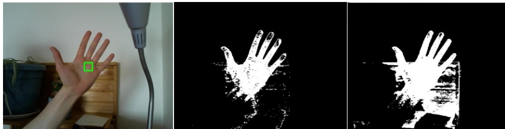
Figure 30 Example Result 4. The left back projection has some occlusion with the wooden shelf. The right back projection has more significant occlusion. More of the hand is selected by the right segmentation but the occlusion is also made worse.
