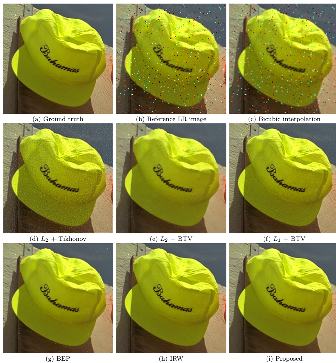
Figure 5.9: Visual comparison of multi-frame super-resolved results from different methods for Hat image with mixed noises.
