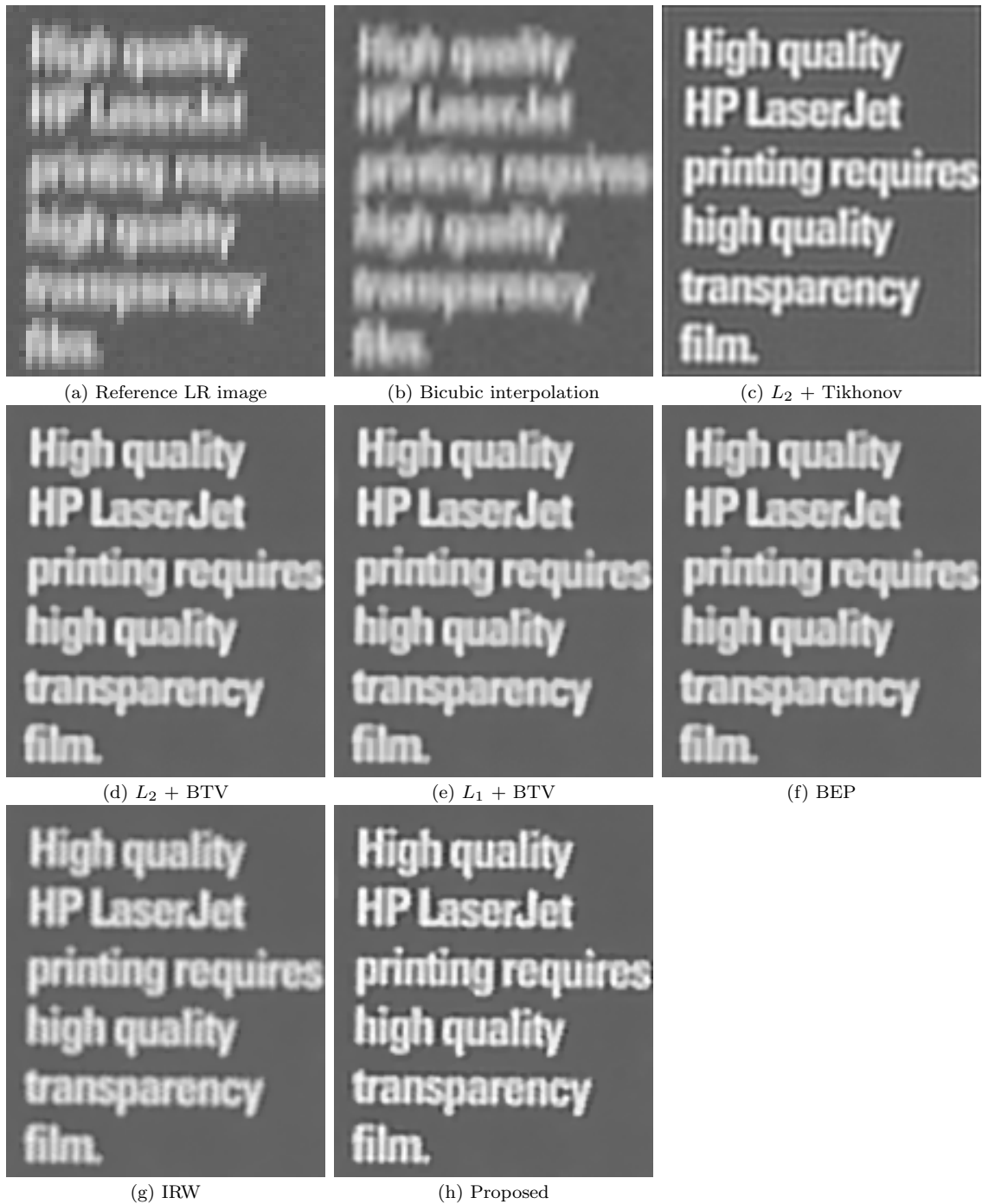
Figure 5.12: Visual comparison of multi-frame super-resolved results from different algorithms for text frames ( r=3 ).
