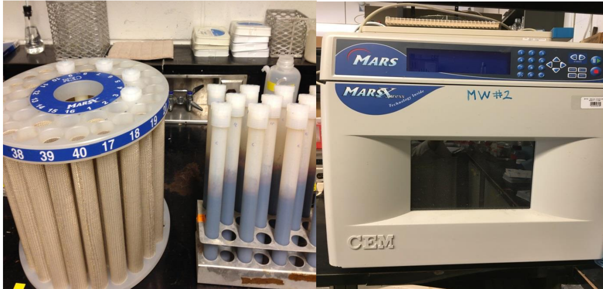
Figure A.8: Teflon-vessels filled and sealed before the MW pretreatment (left), and the Mars X Microwave machine (right).
