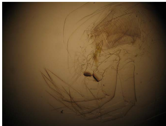
Figure 2.10: Extreme case of an image quality when vignetting is introduced; the light intensity gradually diminishes from the center to the peripheries.
