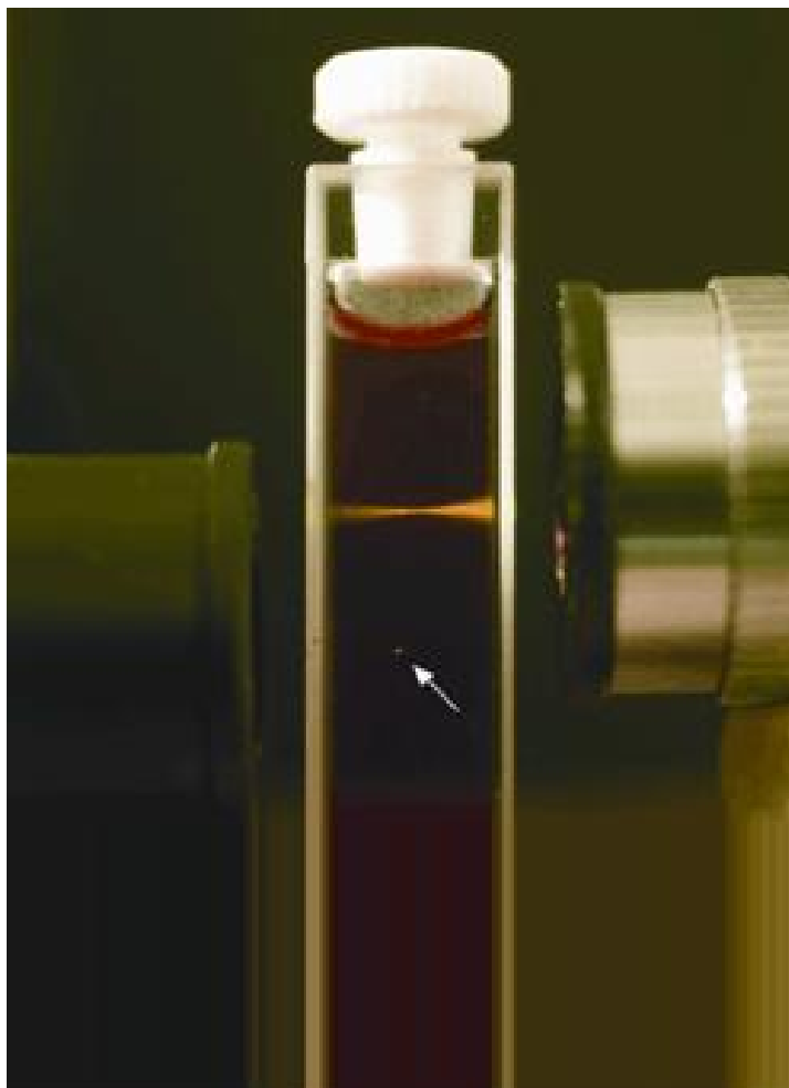
Figure 1.3: This Figure compares the excitation volume of a fluorescent dye (located in a vial) by a multiphoton process (pointed by an arrow, using a multiphoton microscope) to that of a 1-photon excitation process (top, using a confocal microscope). The difference between the interaction volumes associated with the 2 process is clearly significant. For a multiphoton interaction, the excitation of the dye molecules only occurs where the intensity is at the highest and that is at the laser focus, as seen in the picture. This confined interaction is called energy localization, which is a unique property of multiphoton microscopy and gives it its 3D capability. (courtesy of Brad Amos MRC, Cambridge).
