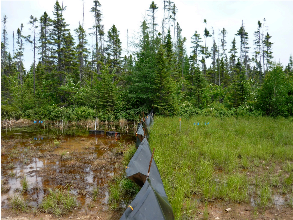
Figure 3.1 Photograph of experimental setup. Twelve wetlands were split in half using an impermeable curtain. One side of each wetland was oversprayed with Roundup WeatherMax® (0.21 or 2.89 mg a.e./L) and the other side was oversprayed with water (control). In this example (PEC 22), the left side of wetland was treated with 2.89 mg a.e./L Roundup WeatherMax® and the right side was treated with water (control).
