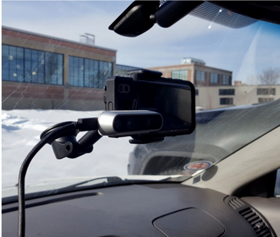
FIGURE 6.1: Thermal camera and its location for data capture.
