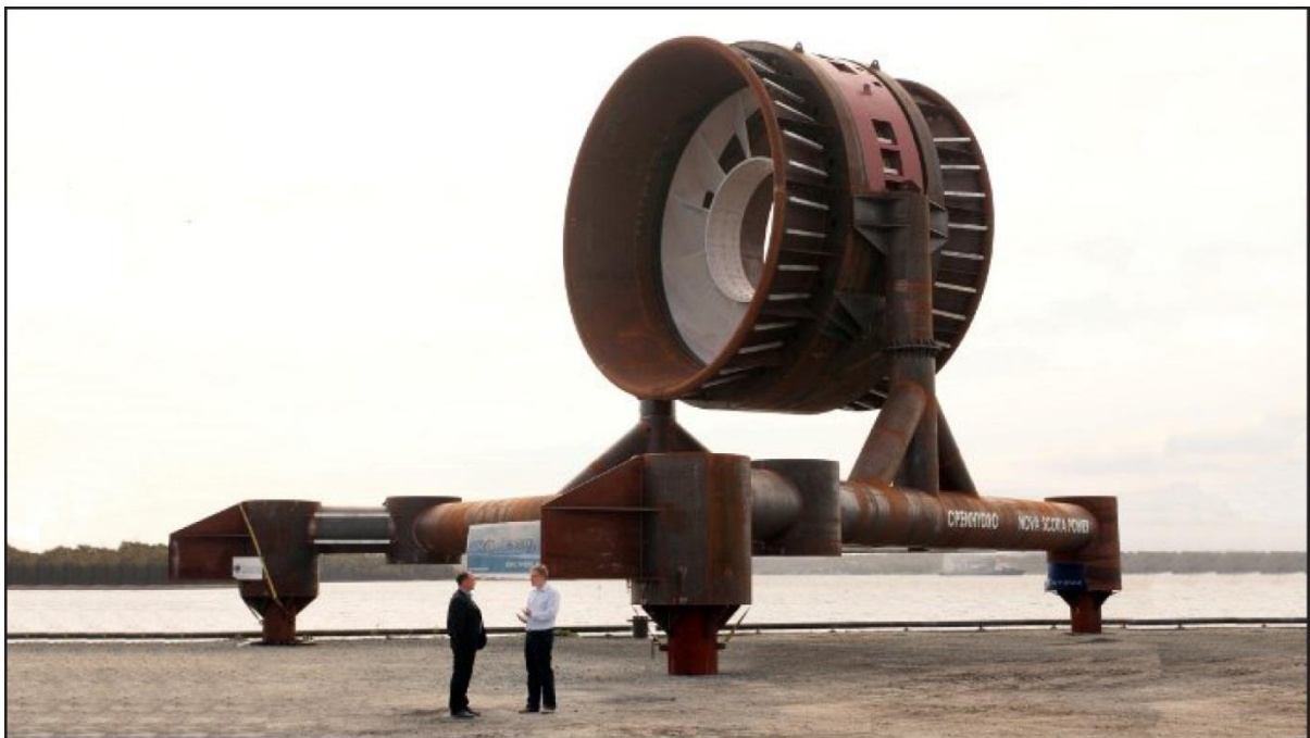
Figure 2.6: In-stream tidal current turbine. (Courtesy of OpenHydro)
