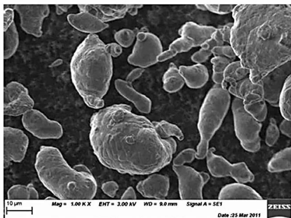
Fig. 5 SEM image of as-received pure aluminum feedstock powder
