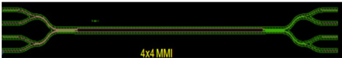
Figure 4.5 Example layout of design mask for a 4 \times 4 MMI coupler. From [79].
