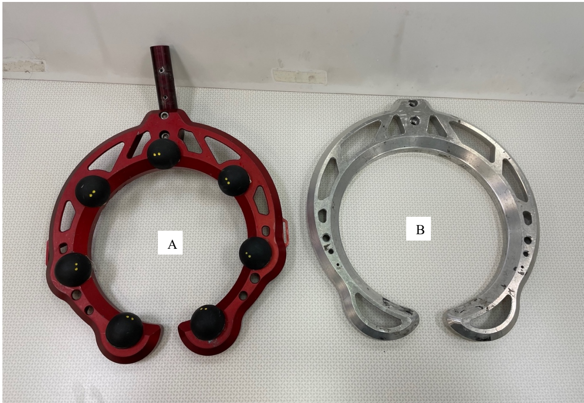
Figure 10. Drop carriages used for head-to-boards impact events.
