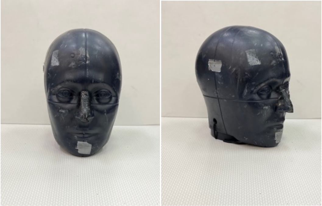
Figure 19. NOCSAE head form, front (left) and front-diagonal (right).
