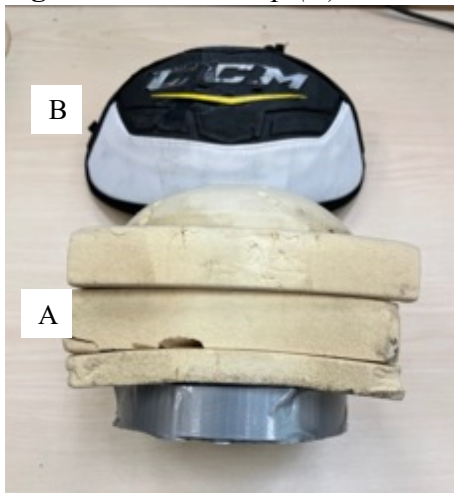
Figure 17. Striker cap (A) and shoulder pad (B).
