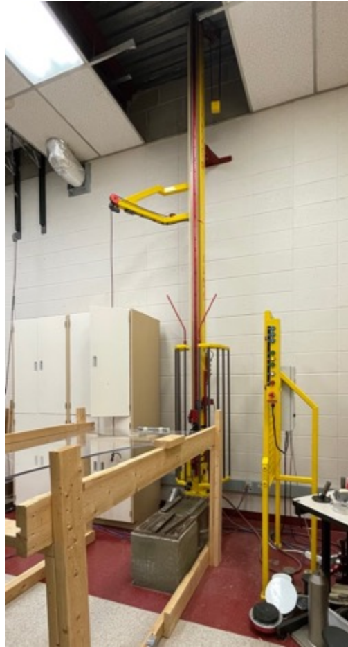
Figure 12. Monorail drop rig setup for head-to-glass impacts.
