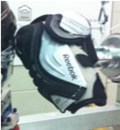
Figure 4.5. Elbow striker used in this study to mimic mass and compliance of an extended elbow strike in ice hockey.
