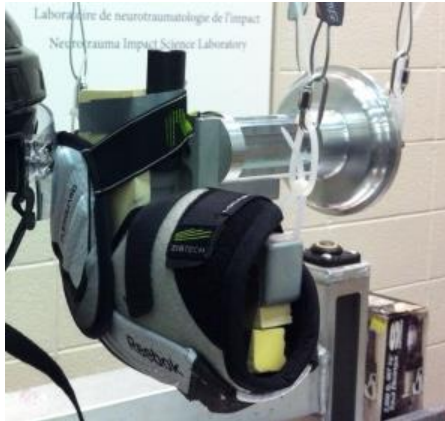
Figure 4.7. Elbow striker used in this study to mimic mass and compliance of a tucked-in elbow strike in ice hockey.
