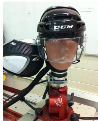
Figure 4.2. Frontal view of the helmeted Hybrid III headform used to represent the struck player.
