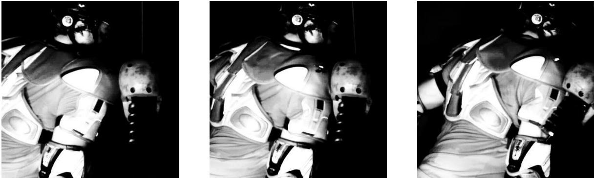
Fig. 3.4. Head linear acceleration history of a shoulder check. The image on the left is at time 0 s (contact), the image at the centre is at time 0.012 s (peak acceleration), and the image at the right is at time 0.030 s (acceleration back to baseline).
