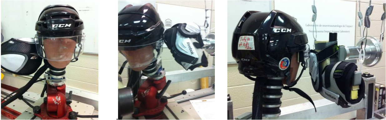
Figure 5.1. Examples of the experimental setup for physical reconstructions of shoulder check (left), extended elbow strikes (centre), and tucked-in elbow strikes (right).
