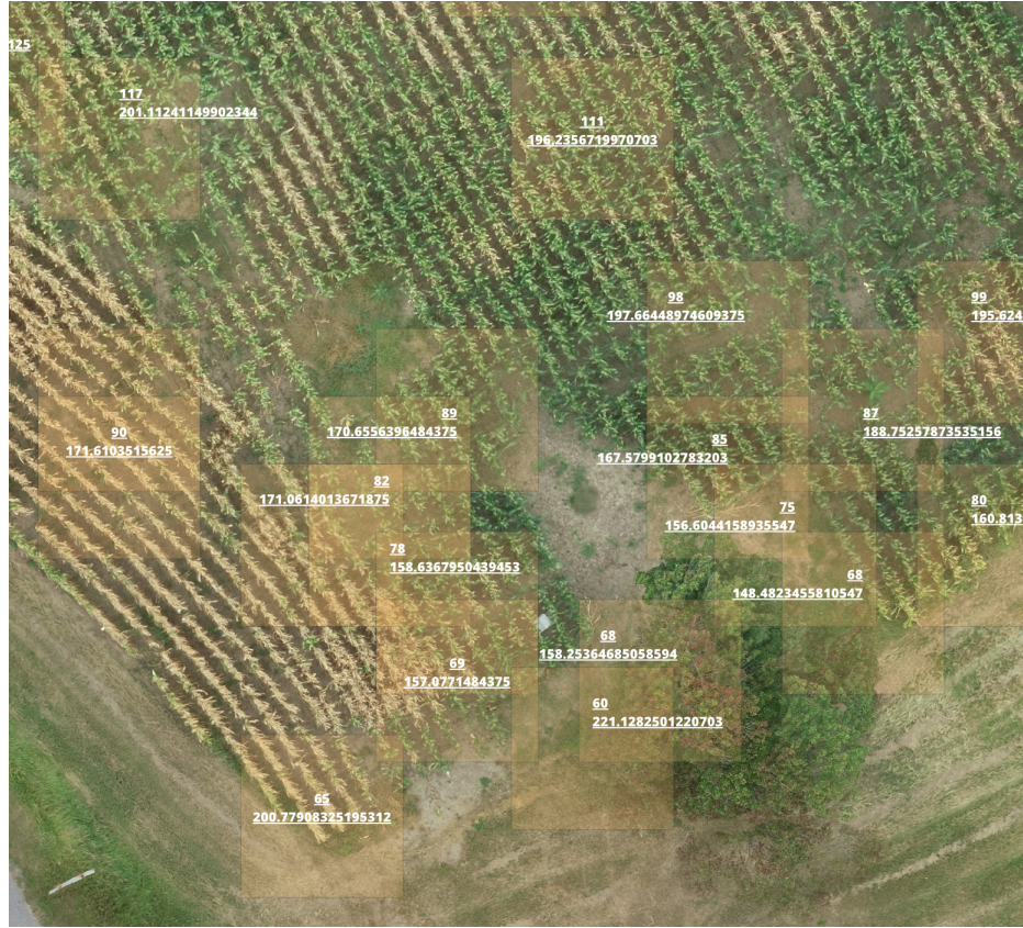
Figure 4.13: The image shows a section of Field 2 with square polygons of size 9X9 m that were extracted for model training. Each polygon displays two values - the top value represents the actual yield, while the bottom value corresponds to the predicted yield.
