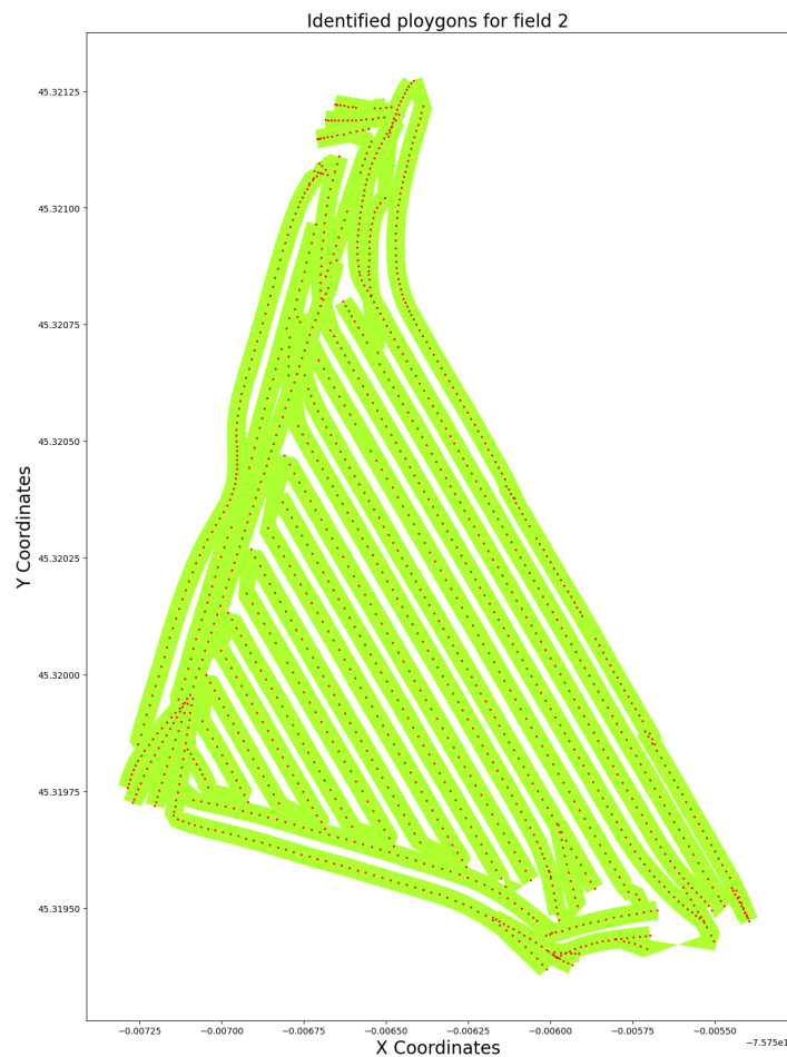
Figure 3.22: The green area represents the identified harvested area in form of a polygon and the red dot represents the actual data point that was captured by the harvester from Demo Field 2
