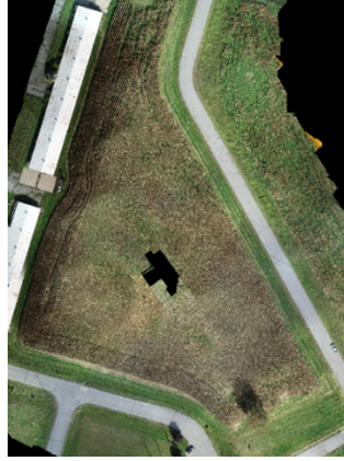
Figure 3.10: Example of an ill-formed mosaic from Field 2 that has missing pixel values
