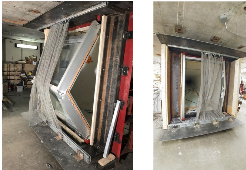
Figure 1 - 1 : Typical curtain wall failure during shock tube tests
