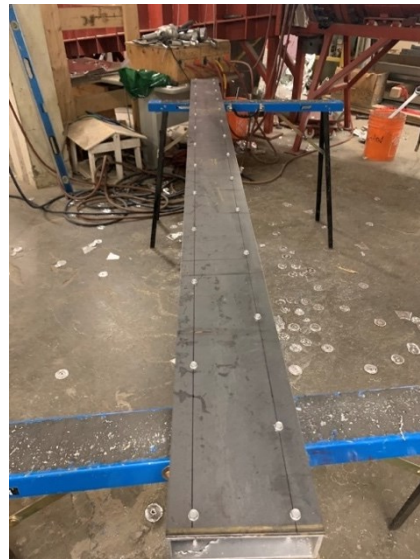
Figure 3 - 22 : Mullion 2H under preparation with initial bolt spacing of 200 mm c/c
