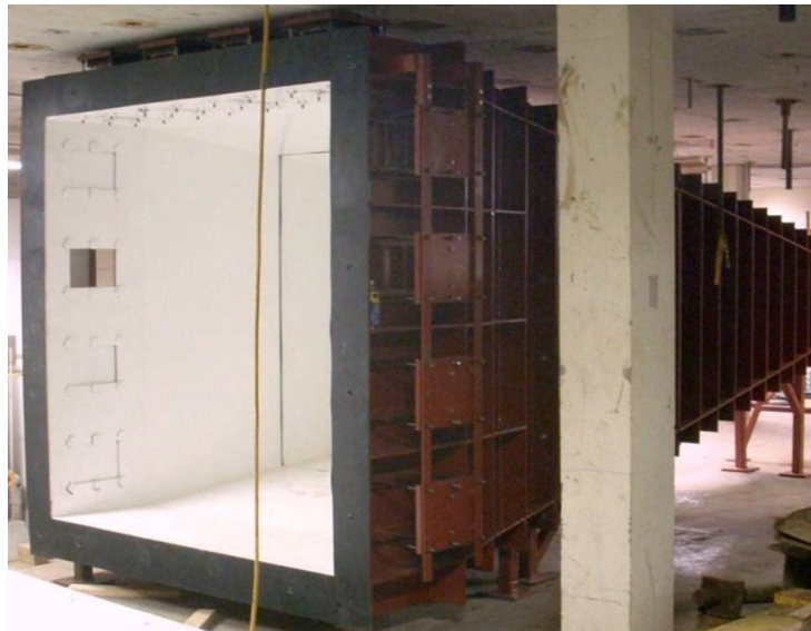
Figure 3 - 5 : Shock tube expansion section opening / vents
