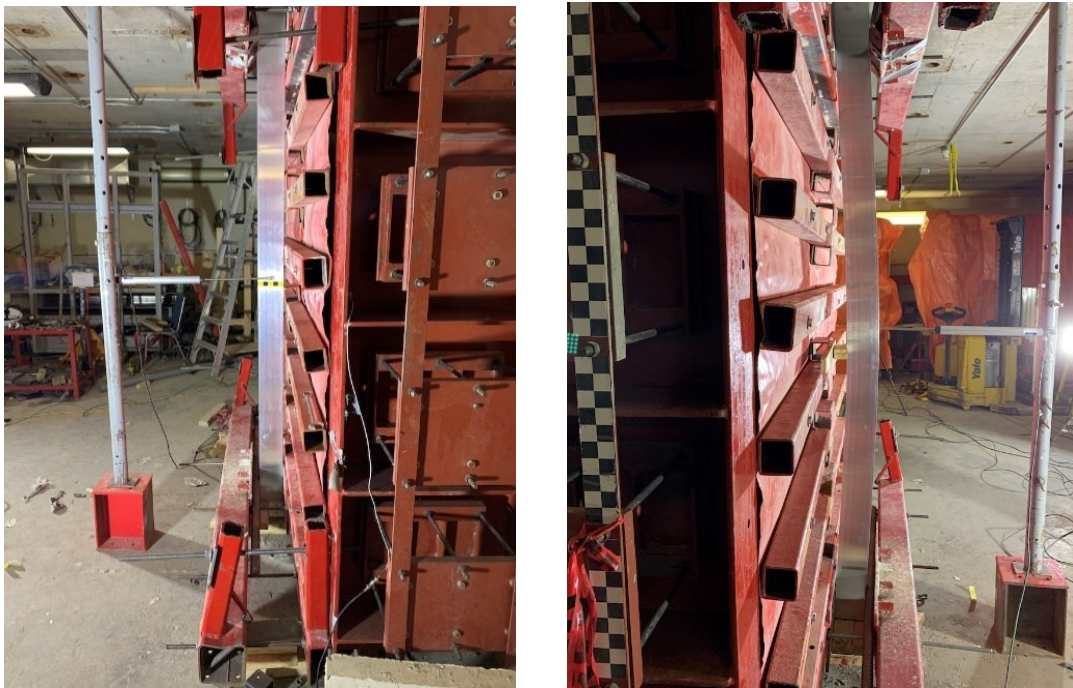
Figure 3 - 30 : Mullion 3 prior to first shot (left) and after first shot (right)
