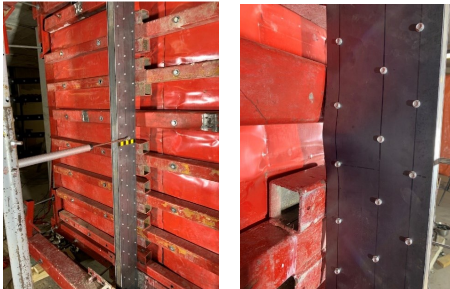
Figure 3 - 32 : Mullion 3H before (left) and after (right) the first shot
