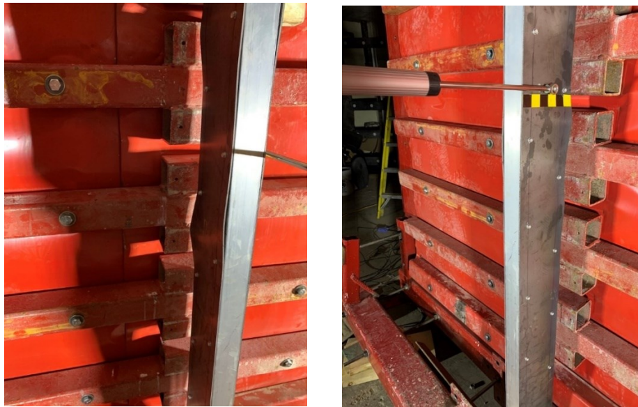
Figure 3 - 24 : Mullion 2H with bolt spacing 200 mm c/c after the first shot
