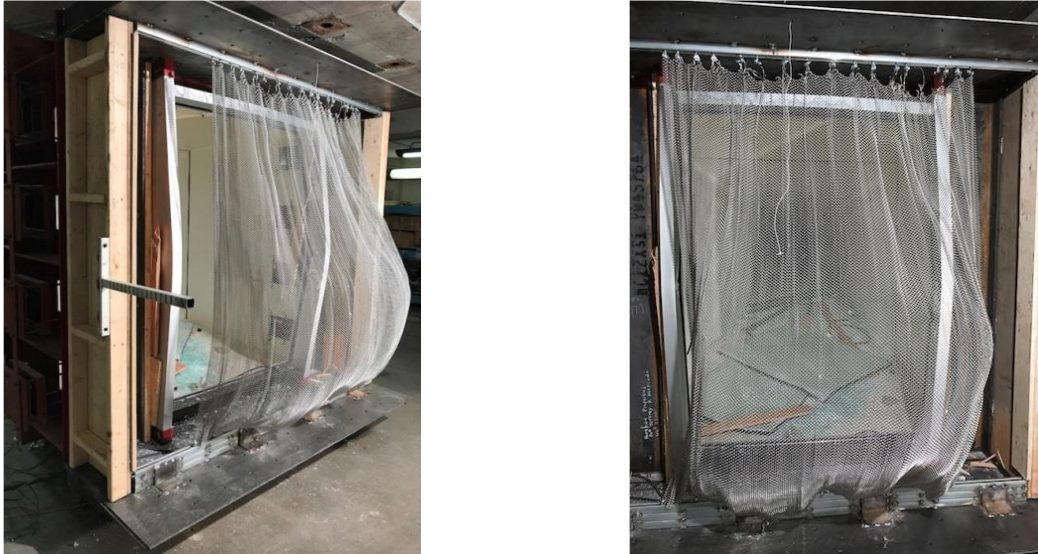
Figure 2 - 10 : Curtain Wall 1 after the test
