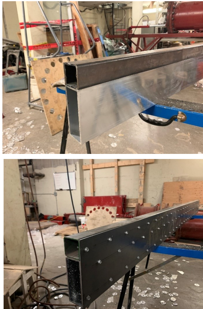
Figure 3 - 3 : Mullion 3H - HSS section on tension flange (left) & side plate bolting (right)
