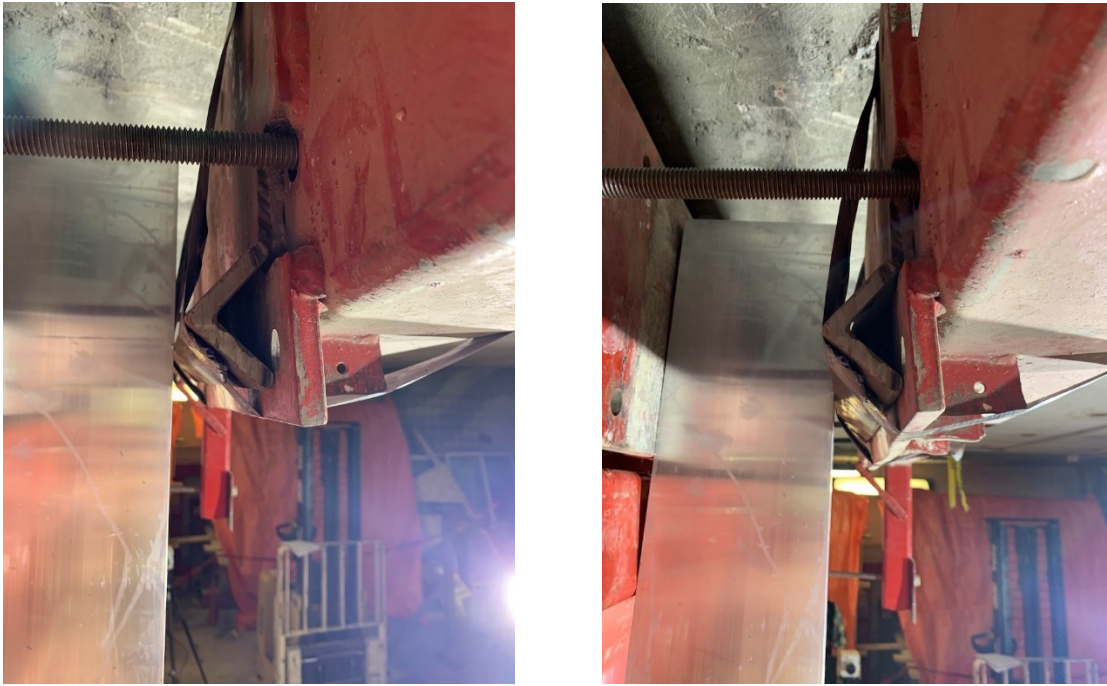
Figure 3 - 8 : Test mullion with simple support assembly
