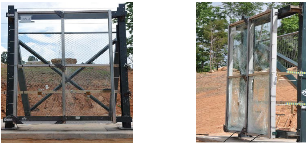
Figure 2 - 15 : Curtain wall specimen before testing (left) and after testing (right)
