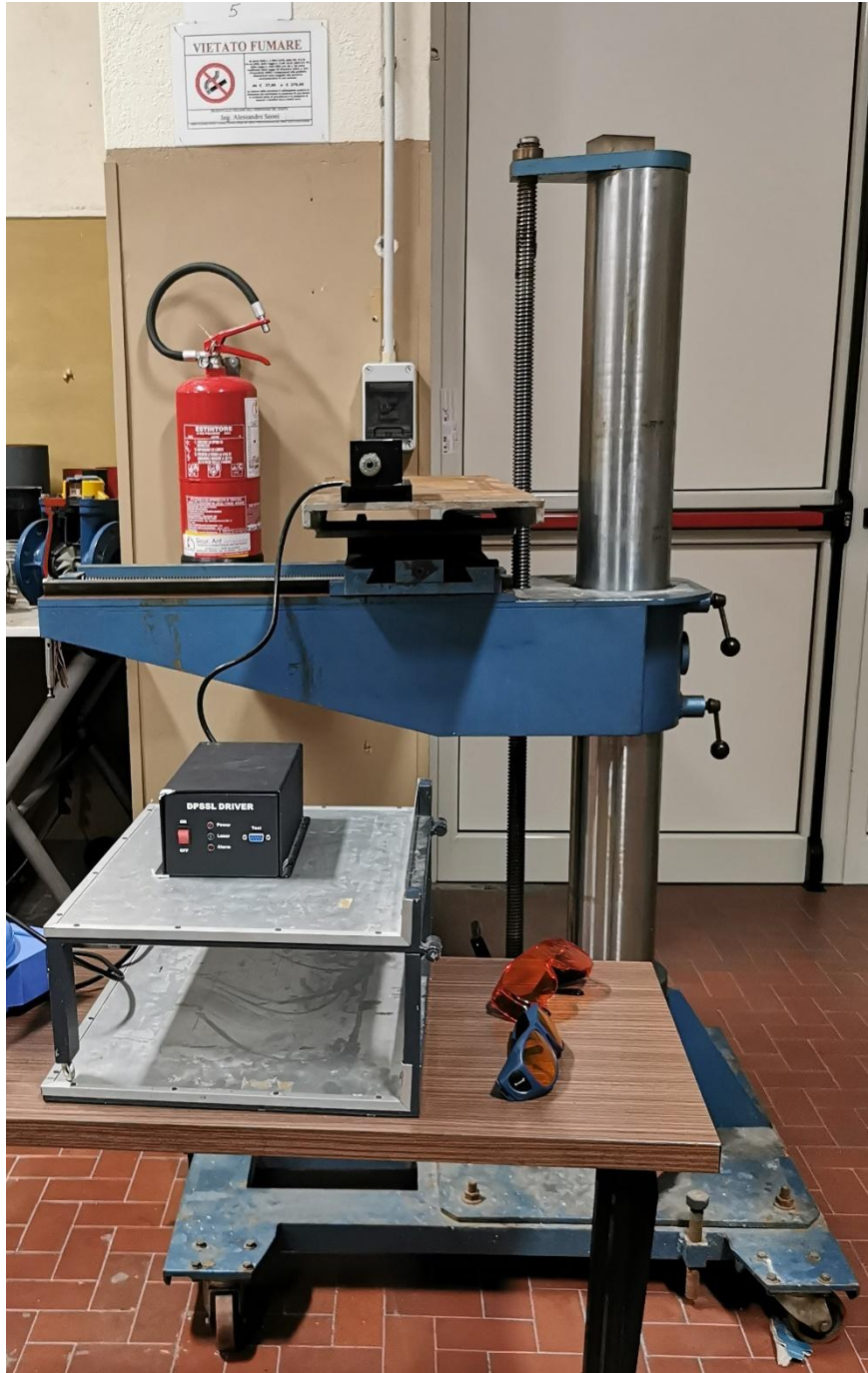
Figure B-6 Tool used to move the laser sheets, showing the laser setup
