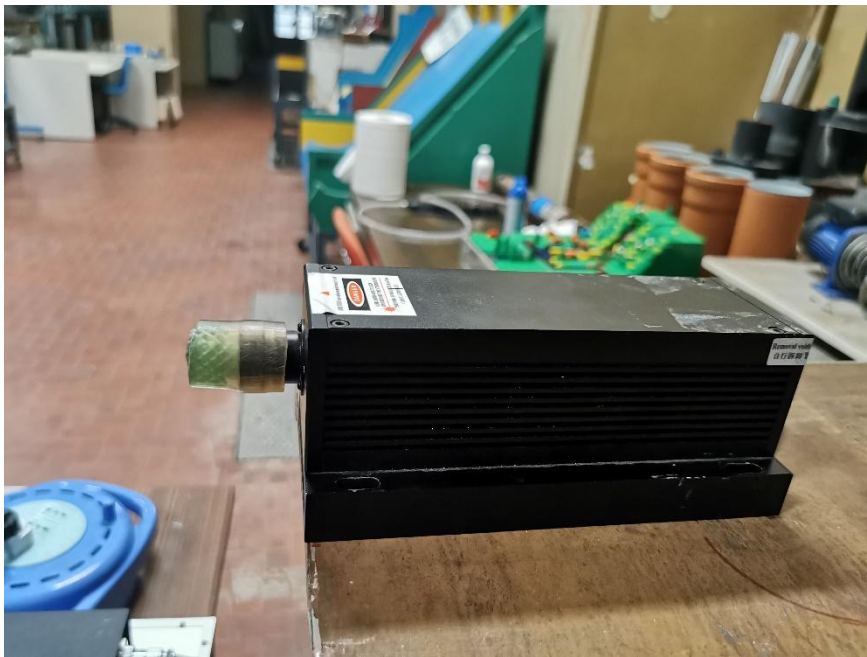
Figure B-2 5-W diode-pumped solid-state (DPSS) continuous green laser
